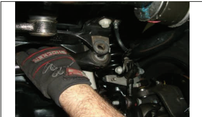
Re-attach trac bar to frame mount and torque to spec.
