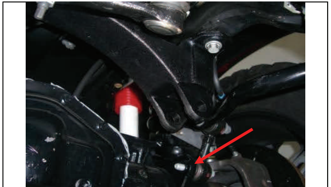
(.05-10) Re-attach and tighten sway bar end links.
