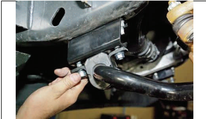
Raise sway bar and attach with new hardware. Leave loose.
