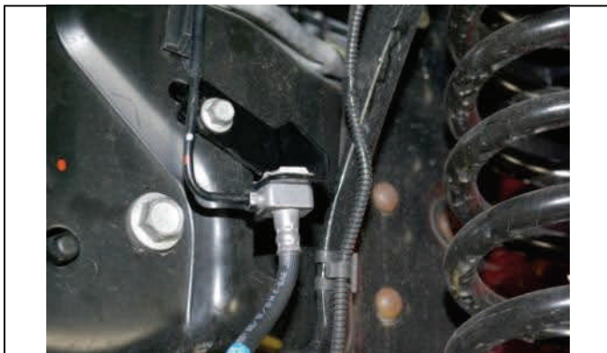
Reinstall block into bracket with retaining clip.
