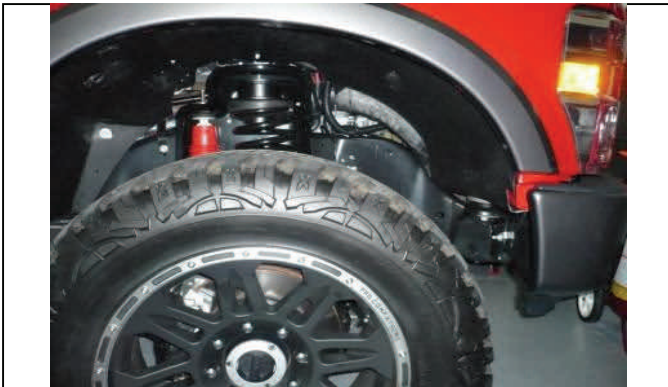
Reinstall wheels/tires, lower vehicle and torque to spec.
