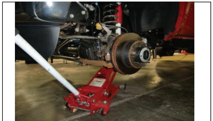
Support front axle with floor jack(s).
