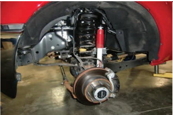
Remove front wheels and tires.
