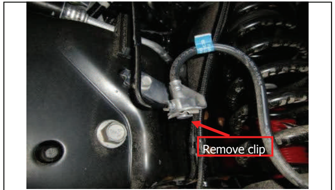
(11-up) models replace OE bracket with new drop bracket.
