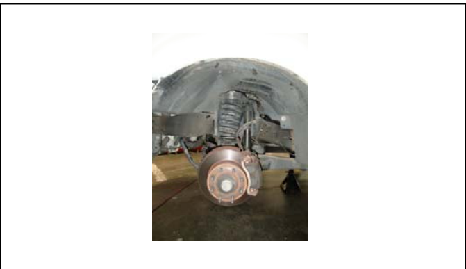
Lift the vehicle off ground and remove the front tires.
