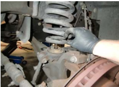
Lower the beam with jack and remove rubber grommet.
