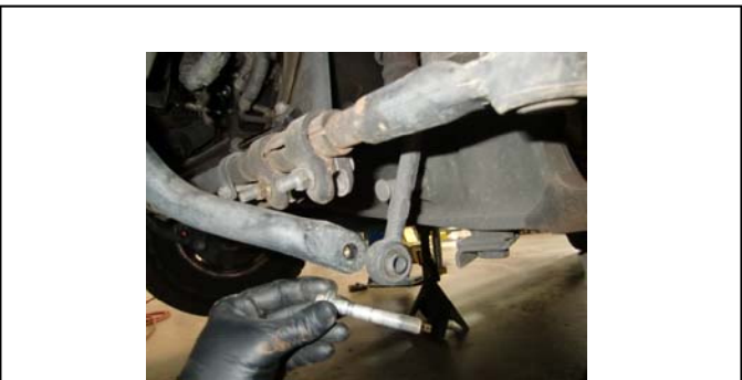
Remove the bolts and twist the sway bar out of the way.
