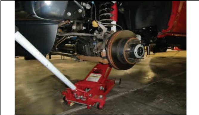
Support front axle with floor jack(s).
