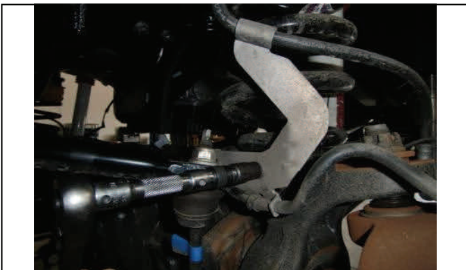
Disconnect brake line support bracket
