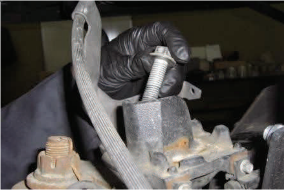
Remove bolt from middle of spring perch
