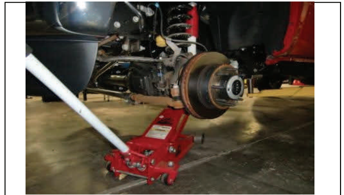
Support front axle with floor jack(s).
