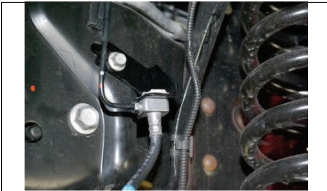
Reinstall block into bracket with retaining clip.
