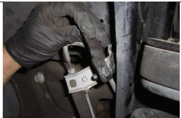
Install drop bracket and attach to frame with OE hardware.
