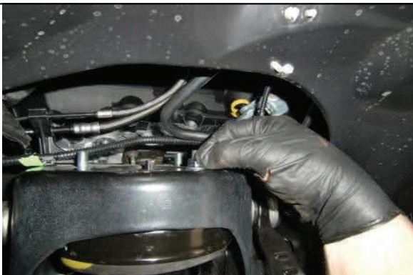
Rotate strut 180 degrees and reinstall with new hardware.
