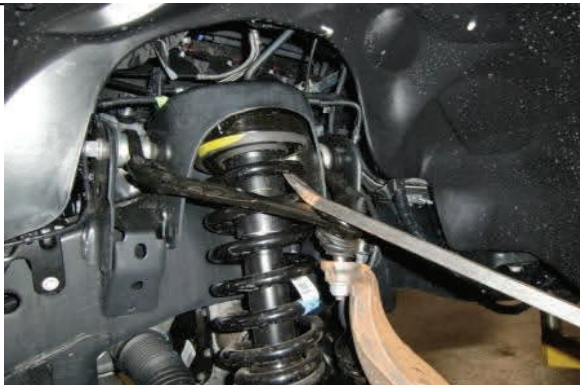
Use jack and pry bar to reattach upper ball joint to spindle.
