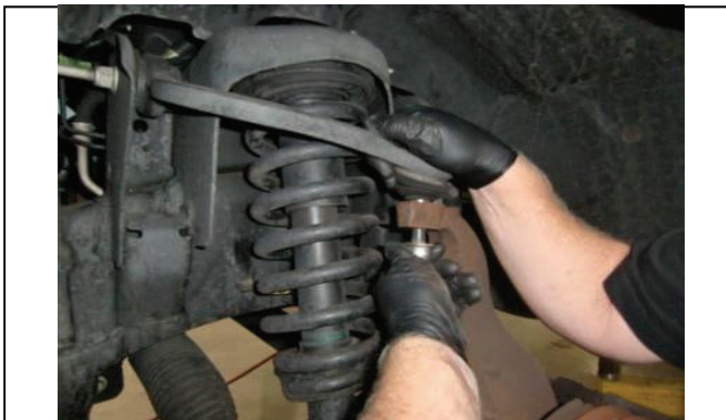
Push down upper control arm and remove ball joint nut
