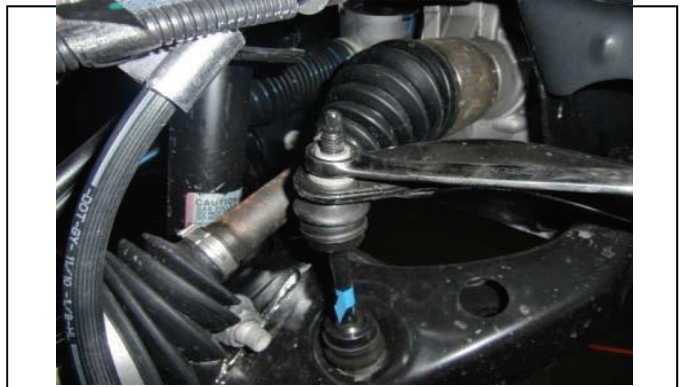
Disconnect sway bar end links on both sides of vehicle
