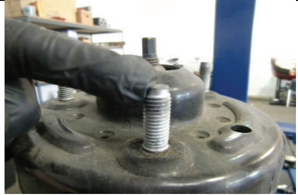
Photo shows tip of studs that need to be trimmed
