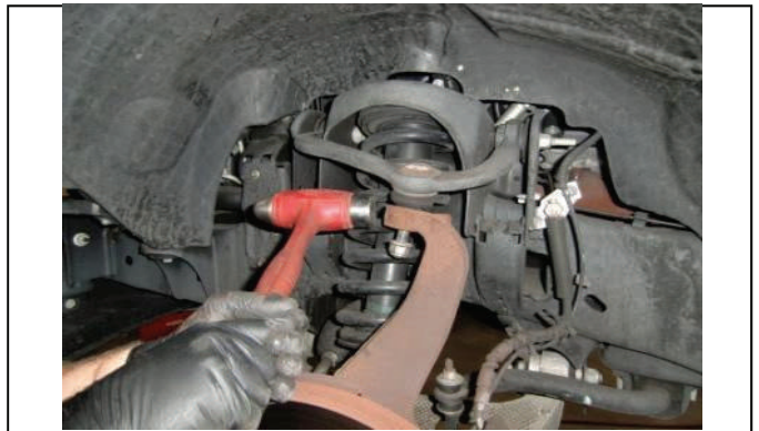
Strike with hammer to disconnect ball joint from spindle
