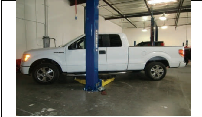
Measure vehicle on level surface and raise by frame
