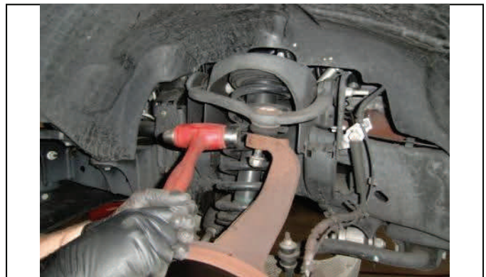
Carefully strike spindle as shown to separate ball joint.
