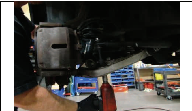
Remove lower sway bar endlink hardware.
