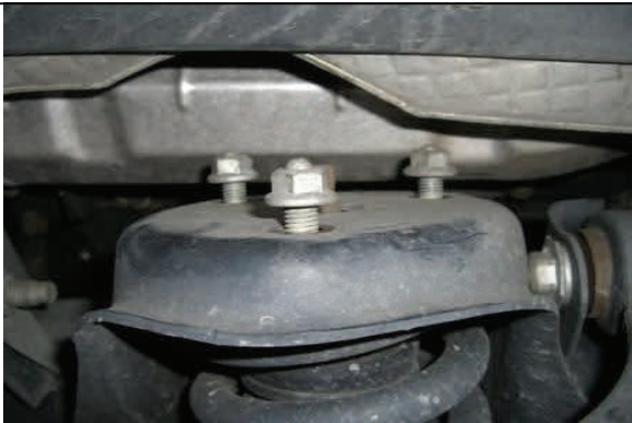
Remove upper strut mounting nuts.
