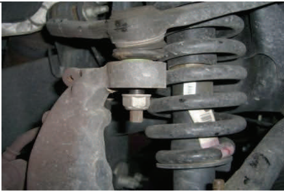
Loosen upper ball joint nut, leave on while breaking loose.
