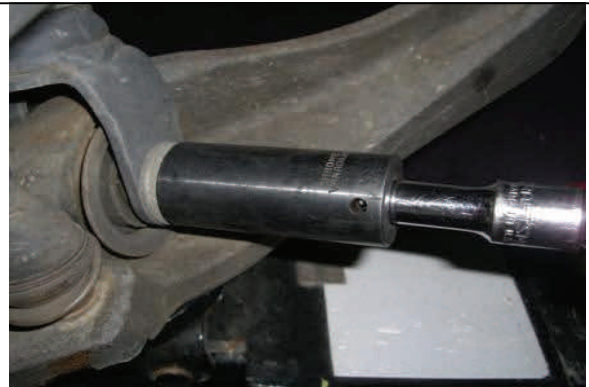
Remove lower strut mounting nut and bolt.
