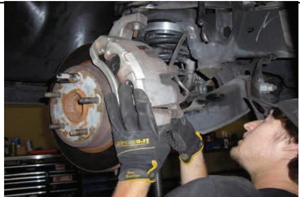
Reconnect brake calipers, sway bar end links, and tie rods.
