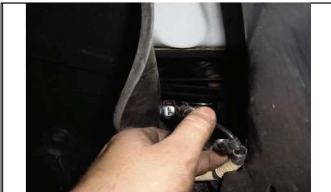
Disconnect ABS line at or behind fender liner.
