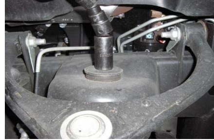
6. Disconnect upper shock mount and bushing.
