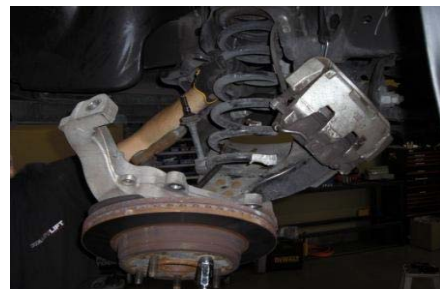
12. Slowly lower suspension and remove coil spring.
