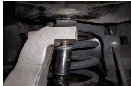
10. Loosen upper ball joint nut and break loose with hammer.
