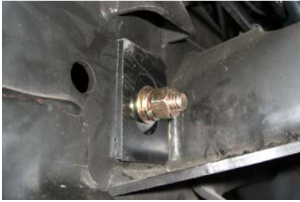
21. Picture shows inner frame bracket & hardware installed.
