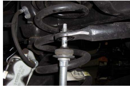
8. Disconnect upper sway bar end links and bushings.
