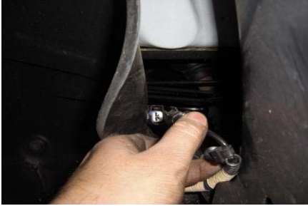
5. Disconnect ABS line at or behind fender liner.
