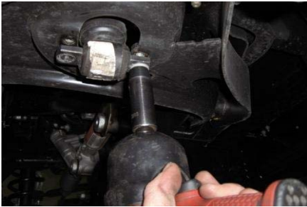
7. Disconnect lower shock mounting bolts.
