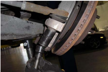
9. Disconnect tie rod end nut and break loose with hammer.
