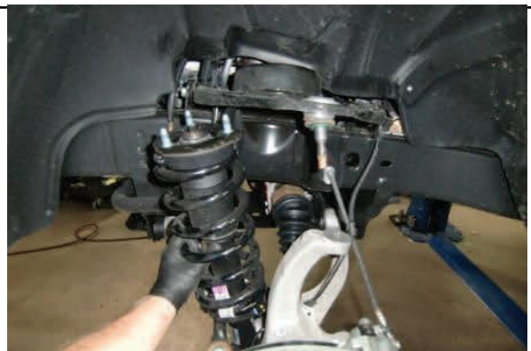
Then, lower strut out of frame and remove from vehicle.
