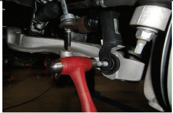
Gently tap lower strut mounting bolt out.
