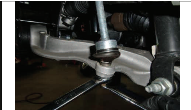
Remove lower sway bar end link at control arm.
