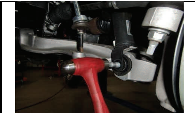
Gently tap lower strut mounting bolt out.
