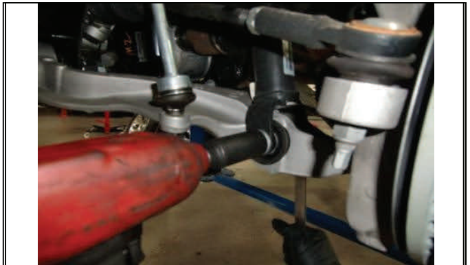
Remove lower strut mounting nut.
