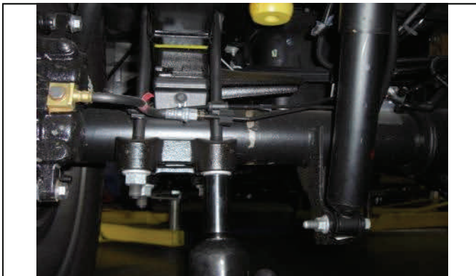
Remove U-bolt nuts and axle mounting plate.
