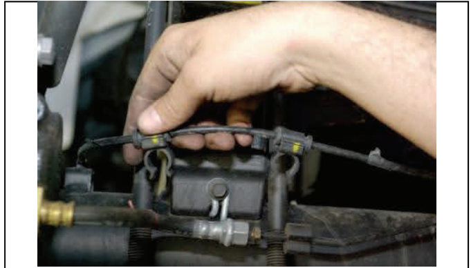
Vehicles with ABS/TC remove clips from U-bolts.
