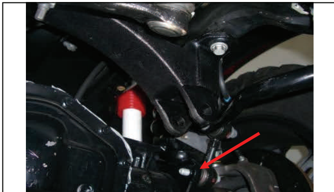
(05-10) Re-attach and tighten sway bar end links.
