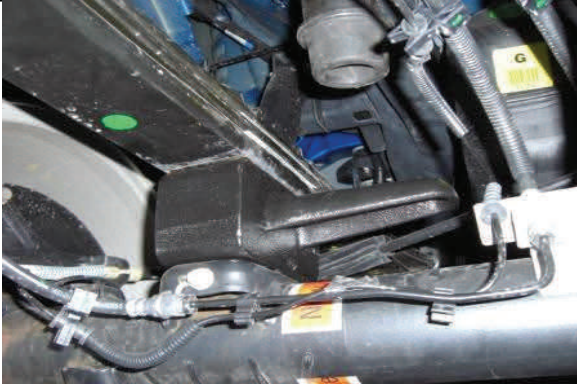
Raise axle and center on locating pins in leaf spring.
