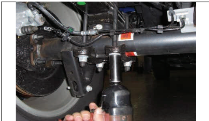
Loosen and remove factory u-bolt hardware.
