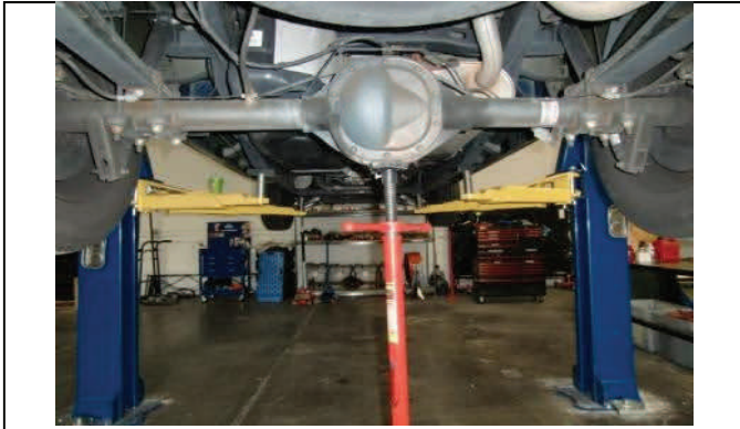
Raise vehicle at frame and support axle with jack
