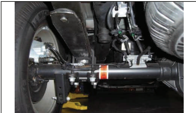
View of 2WD rear axle and leaf springs.
