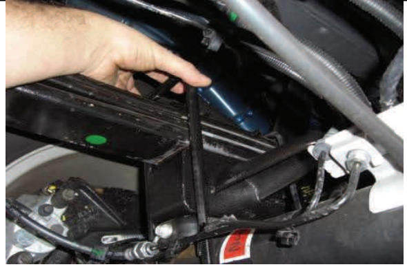
Place new longer u-bolts over leaf spring and axle.
