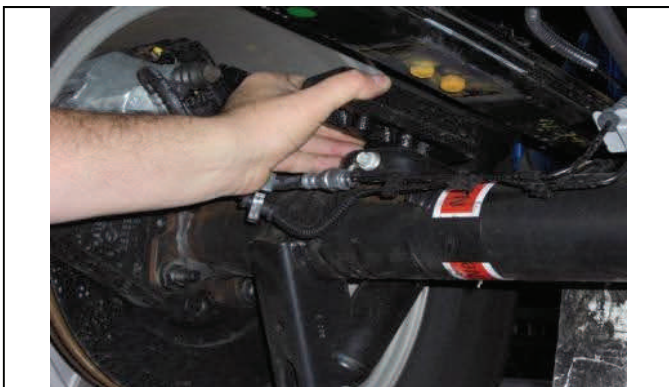
4WD only: Lower axle enough to remove factory block.
