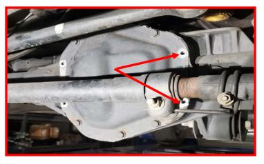
Differential ID tag shown installed on the drivers side using the (2) factory bolts.
