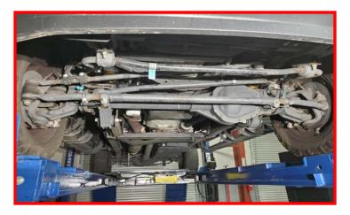
Remove the (2) middle bolts on the passenger side of the differential cover and retain the factory hardware. Save the differential ID tag for the step below.
