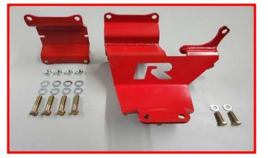
Install the center stabilizer bracket using the supplied  $3/8'' \times 1-1/4''$  hex head bolts and 3/8" flat washers. Tighten bolts enough to secure the main body to the passenger side of the differential but do not tighten completely at this time.
