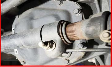
Locate the center stabilizer bracket and rear axle clam shell of the dual steering stabilizer kit and the following hardware:
