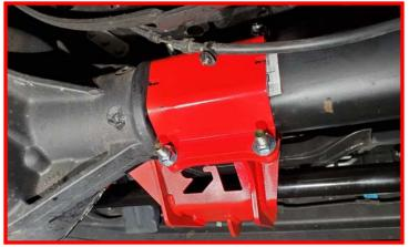
Install driver side drag link bracket using the supplied M8 x 75mm hex bolts, M8 lock nuts, M10 x 90mm carriage bolts and M10 lock nuts. Do not fully tighten at this time.
