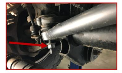
Using a hammer/Air hammer, hit side of track bar to unseat taper as pictured.
