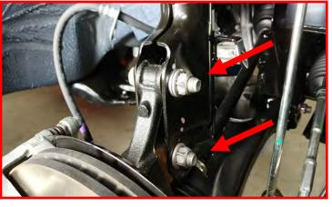
Locate the ReadyLIFT front strut extension. These are driver and passenger side specific and have a D and P etched into the top. Passenger side shown. Install to the top of the strut using the factory hardware. Torque to 30 ft-lbs.
