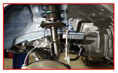
Raise the knuckle up and install into the strut body. Install the cam bolt into the upper hole and the remaining bolt into the lower.
