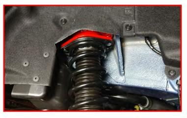
Raise the lower control arm into place and install the lower strut hardware. Do not tighten at this time. Use the jack and raise the lower control up to set pre load on the strut. Install the lower knuckle bolt. Torque to 95 ft-lbs.
