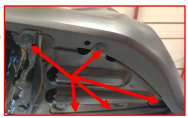
From the edge of the bumper cover closest to the wheel well, measure to the front 3/4" and mark a line as shown. There is a mold line for the forward cut you can follow. Use a suitable cutting tool and trim this lip off. You will be removing the last mounting hole and trimming this area allows the plastic to slide forward.
