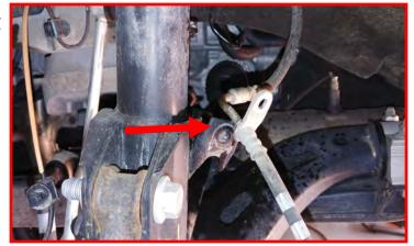
Remove the ABS harness clip at the strut body. Let hang out of the way. Remove the strut to knuckle bolts. The bolts are specific to upper and lower mounting locations and direction of install. The upper is a cam bolt, while the lower is a standard bolt. Make sure to note their orientation for reinstallation later.
