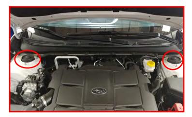
Locate the ReadyLIFT front strut extension. These are driver and passenger side specific and are etched with a D and P. Passenger side shown. Install to the top of the strut using the factory hardware. Torque to 30 ft-lbs.
