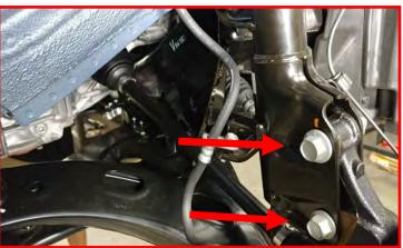
The cam bolt has lines that correspond to a notch on the strut body (paint marked for picture clarification). You will rotate the cam bolt until the lines are facing the inside of the vehicle. Line up the last line with the notch. This sets max negative camber. Torque both bolts to 95 ft-lbs. Final adjustment and torque to be set by the alignment tech.
