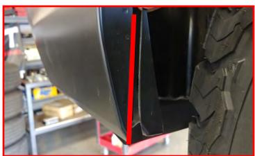
Once the corner is reached, trim the remaining lip to the new inner liner location. This remove the last little edge that can catch on larger tires.
