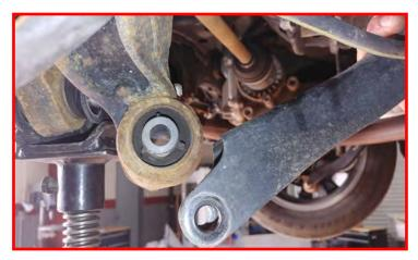
Loosen but do not remove the lower control arm bolt at the subframe. Remove the lower strut bolt on the lower control arm and the control arm bolt at the knuckle.
