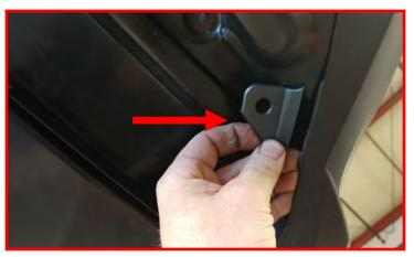
The inside edge clip holes can now be lined up and drilled out. Once done, reinstall using the previously removed clips.
