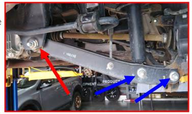
Lower the control arm down and remove the strut from the vehicle and let the control arm hang.
