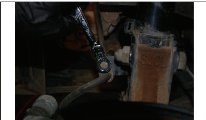
Unbolt brake line from strut
