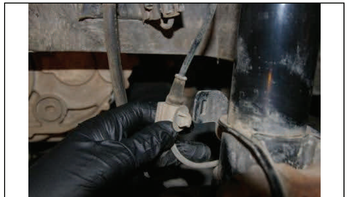
Unclip all ABS lines mounts on strut and at the frame
