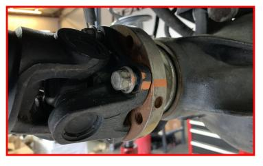
Remove the front drive shaft from differential.
