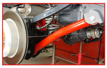
Install the brake line bracket to the axle using the factory hardware. Torque to 5 ft -lbs.
