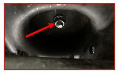
Using the manufactures suggested install instructions, Install replacement performance shocks using factory hardware on top frame mount and provided M12 bolts, washers and nuts.
