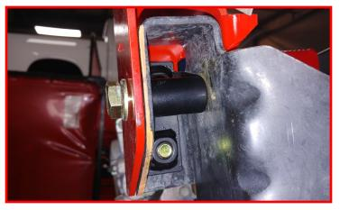
Install track bar into replacement track bar bracket using factory hardware. Do not tighten at this time.
