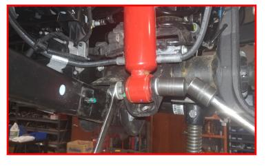
Lower the axle enough to remove the springs.
