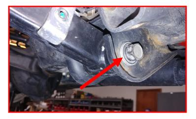
Remove the front shock from vehicle at this point and discard. Retain factory hardware.
