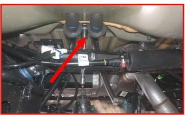
Remove the rear brake line bracket at the axle and frame rail.
