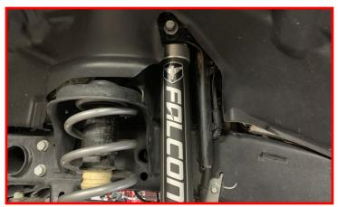
Install the 10" replacement end links to the sway bar using supplied 1/2" bolt, fender washer, flat washer and nut on the sway bar. Be sure to install the fender washer to the outside of the end link. Install the axle side of end link using factory hardware. Torque to 45 ft-lbs.
