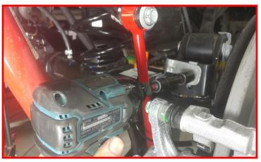
Install the ReadyLIFT brake line bracket to its corresponding side using the provided  $1/4'' \times .75''$  bolt, washers and nut. Gently rotate/bend the metal brake line until you can line up the locking tab and bolt hole. Install using the factory hardware. Torque all to 5 ft-lbs.
