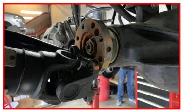
Remove the lower heat shield bolt from the front upper control arm pocket at the frame. Retain hardware for reassembly.
