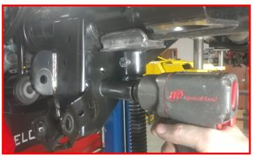
Loosen the rear track bar at the axle and frame. Remove axle bolt only and let track bar swing out of the way.
