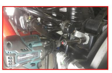
Remove the rear lower control arms at the axle and frame. Retain factory hardware.
