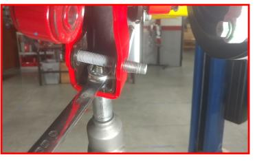
Install the ReadyLIFT brake line bracket to its corresponding side using the provided 1/4" x .75" bolt, washers and nut. Gently rotate/bend the metal brake line until you can line up the locking tab and bolt hole. Install using the factory hardware. Torque all to 5 ft-lbs.
