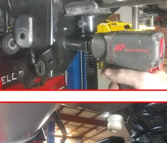
Lower the axle enough to remove the stock spring and rubber isolator. Install the ReadyLIFT spring and factory isolator. Raise the axle enough to hold the springs in place.
