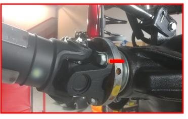
Remove the front drive shaft from differential.
