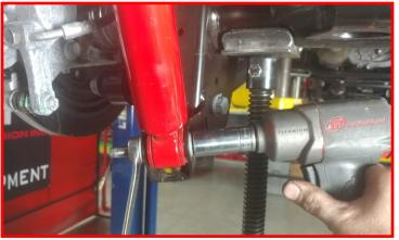
Remove the rear lower sway bar end link from the axle.
