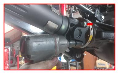
Lower the axle enough to remove the springs. Make sure to not over extend the brake lines or any other electrical harnesses. Insert the front bump stop 3/8" x 1.75" Allen bolt into the front bump stop. Insert the front bump stop into the coil spring.
