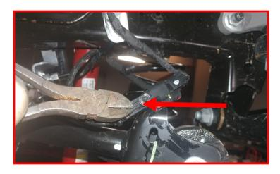
Remove the sway bar end links from the axle. Save the hardware.
