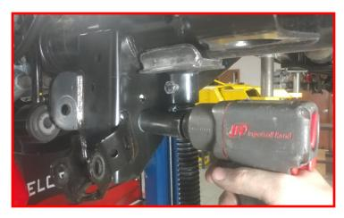
Loosen but do not remove the rear track bar at the axle and frame.
