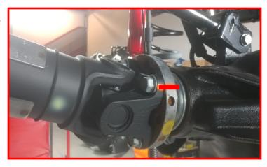
Remove the front drive shaft from differential.
