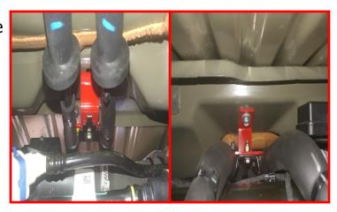
ELECTRIC LOCKER EQUIPPED MODELS ONLY: Connect the electrical connector to the pumpkin and run the harness next to the diff vent tube. Clip all remaining clips to the diff vent tube.
