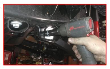
Remove the lower heat shield bolt from the front upper control arm pocket at the frame.
