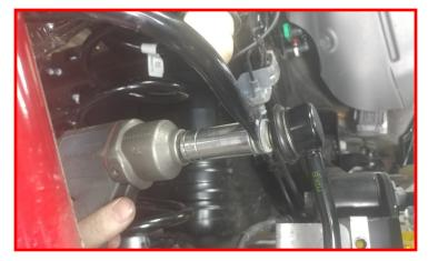
Loosen but do not remove the rear upper control arms at the axle and frame.
