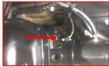
ELECTRIC LOCKER EQUIPPED MODELS ONLY: Remove the two harness clips from the frame cross member. You can clip these off the wire harness but is not necessary.
