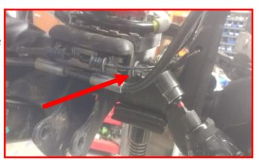
Install the provided 3/8" serrated flange nut to the 3/8" Allen bolt from the under side of the spring perch. Torque to 35 ft-lbs.
