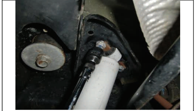
Next, remove rear upper shock bolts.
