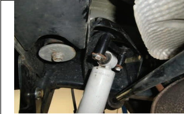
Install upper shock extensions with provided hardware.
