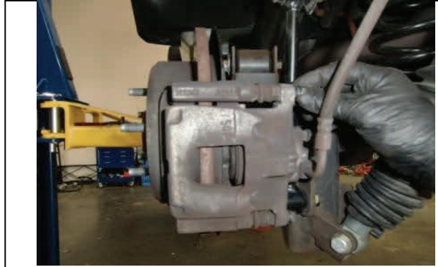
Reattach rear brake calipers and tighten to spec.
