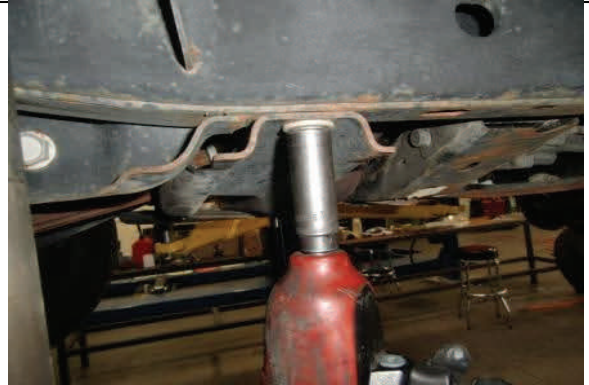
Reinstall front transfer case skid plate bolts.
