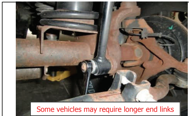
Reattach front sway bar end links .
