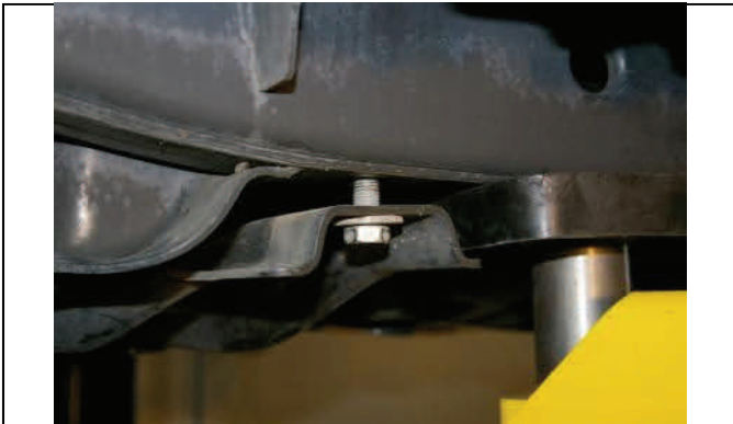
Remove (2) front transfer case skid plate bolts.
