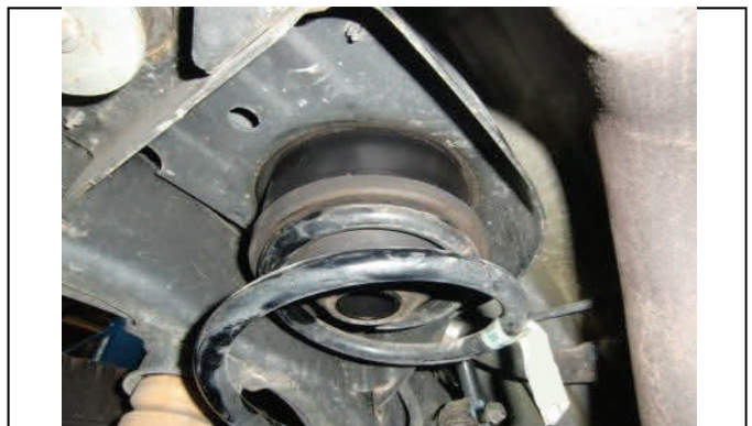
Reinstall OE isolator and spring back into vehicle, raise axle
