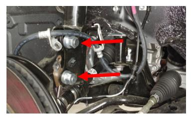
Install the tie rod end to the knuckle using the factory hardware. Torque to 65 ft-lbs. Line up the cotter pin hole with the slots in the castle nut. Install the cotter pin.
