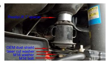
Use a 10mm wrench to remove the driver side rear cradle stud. Add one of the Readylift 1" aluminum spacers. Use the provided hardware M16 bolt, washer, and laser cut 2" washer to reattach. After one side is complete, repeat this same steps on the passenger side. Snug these bolts but do not tighten. After all four bolts are installed torque the M16 bolts to 90 ft-lbs.
