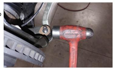
Remove the sway bar end link from the strut. Let hang out of the way.
