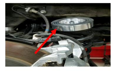
Reposition the spring assembly, so the spring spacer nipple aligns with the hole on the vehicle frame.
