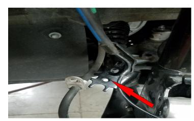
Reinstall the ABS senor to the steering knuckle, use the factory hardware torque to 5 ft-lbs. Push to clip the ABS plastic bracket to it's original location on the lower strut assembly.
