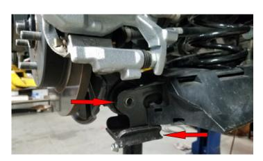
Reattach the brake line using the factory hardware torque 10 ft-lbs.
