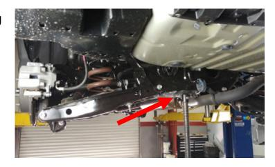
Remove the bolt that holds the brake line to the control arm.
