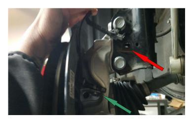
Install the ReadyLIFT sway bar bracket to the strut using the provided M12 bolts, washers, and nuts. Install the sway bar end link to the bracket using the factory hardware. Torque all to 45 ft-lbs.
