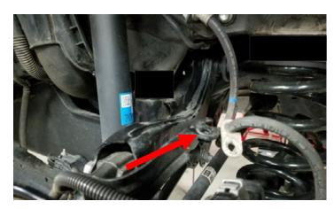
With the suspension cradle supported, remove the front two cradle bolts and the rear cradle nuts. Lower the cradle 1"using the rear cradle studs as an alignment guide.
