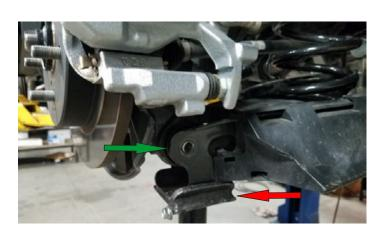
Add the ReadyLift spring spacer to the top of the spring. Use the ruber isolator between the spring and spacer.
