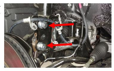
Remove the 3 upper strut mount hardware on the strut tower in the engine compartment. Use of a helper is recommended to hold the strut while removing from the strut tower.
