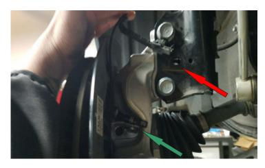
Remove the tie rod end nut. Strike the tie rod end boss with a dead blow hammer to dislodge the taper. Let hang out of the way. This allows you to turn the knuckle free of the rack and pinion to remove the strut.
