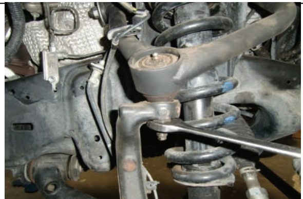
Raise suspension and reattach upper ball joint to spindle.
