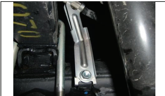
Remove brake line bracket bolt from axle tab.
