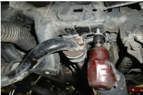
Disconnect sway bar at the frame mounts.
