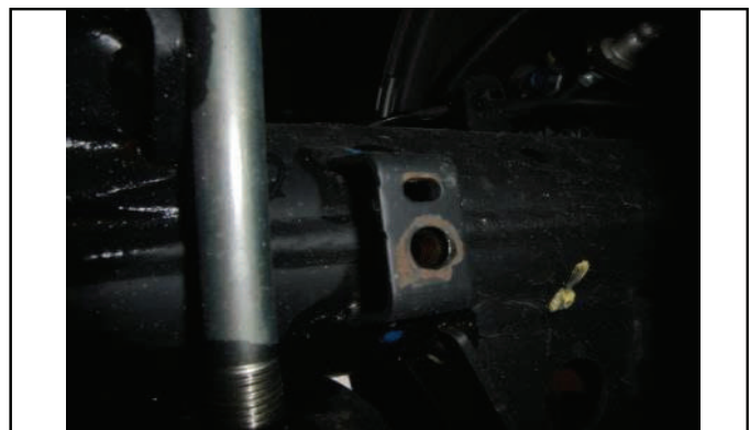
Axle tabs and brackets are different on either side.
