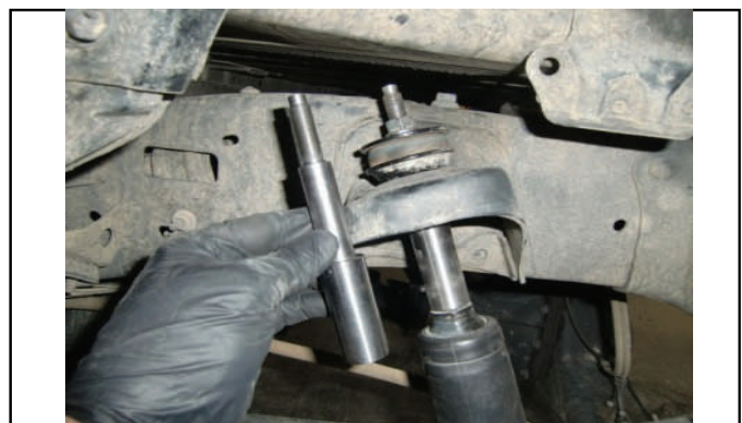
Install provided upper shock extension as shown.
