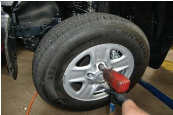
Remove wheels/tires from vehicle.
