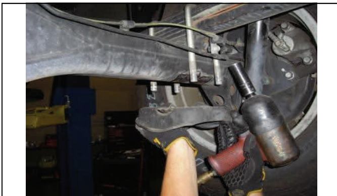
Remove u-bolt nuts and lower plate.
