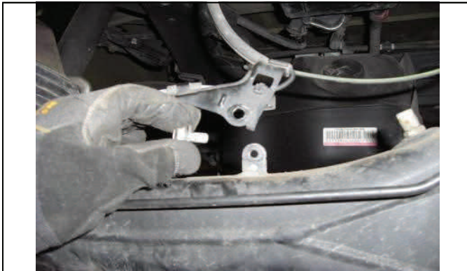
Disconnect ABS wiring brackets from axle.
