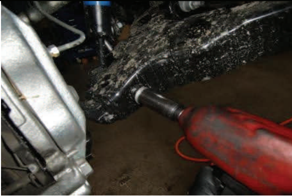
Reattach and tighten lower strut mounting hardware
