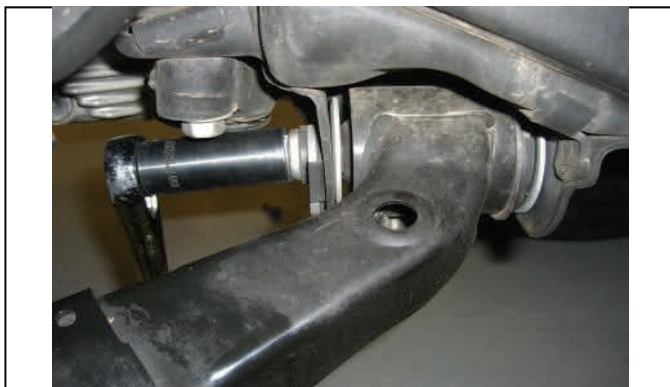
Loosen both lower control arm pivot/alignment bolts
