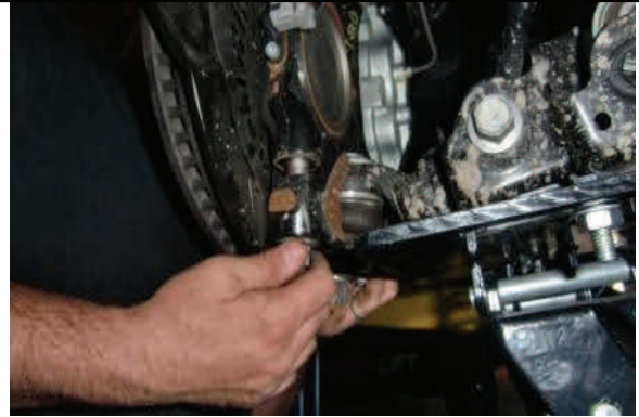
Raise lower control arm, reattach (2) ball joint mounting bolts
