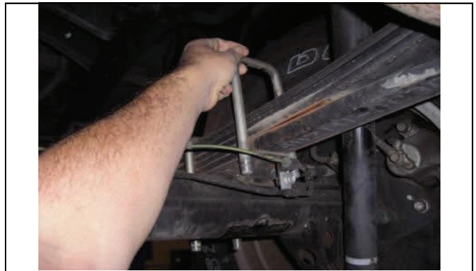
Carefully lower axle and remove u-bolts
