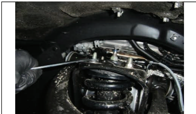
Remove upper strut mounting hardware
