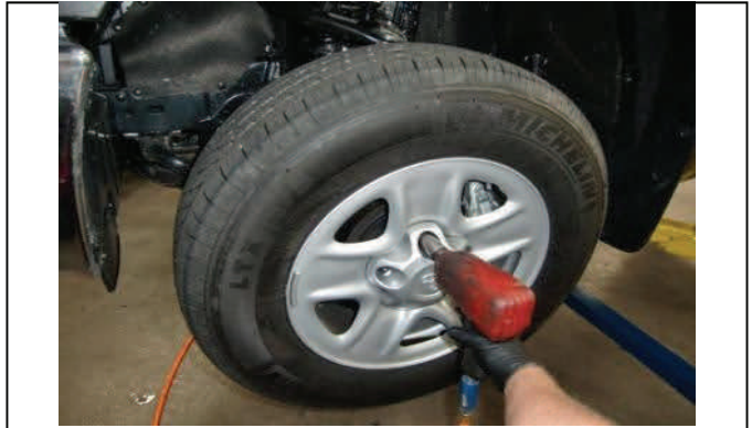
Remove front wheels/tires
