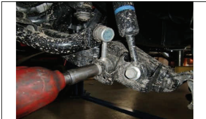
Disconnect lower sway bar end links
