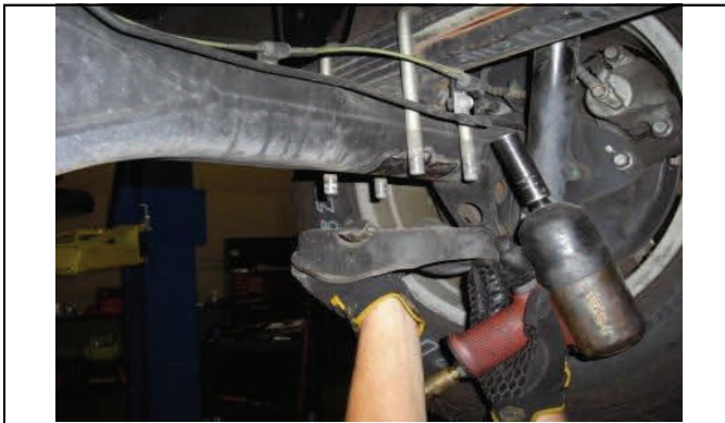
Remove u-bolt nuts and lower plate.
