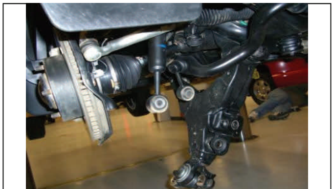
Swing down lower control arm and remove strut
