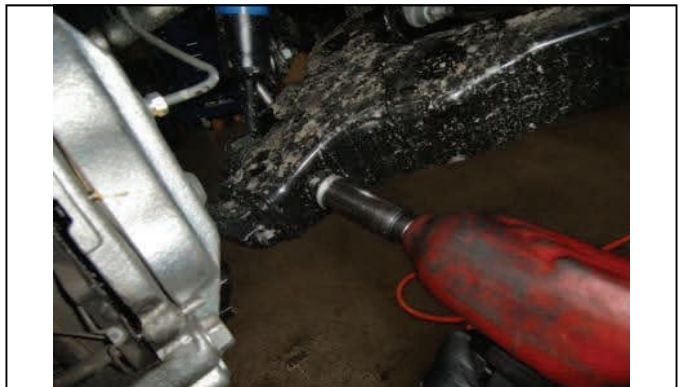
Remove lower strut mounting hardware
