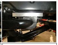
6. Sway bar spacer properly installed.
