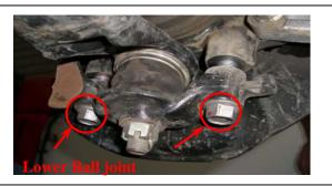
3. Loosen, don't remove the 19mm lower control arm nut and bolt, Remove the 19mm lower ball joint bolts.
