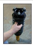
6. Reinstall the strut assembly in its stock location. Leave the three upper strut mounting nuts loose Raise the lower control arm and install the lower strut mounting bolt and nut. Use a floor jack to raise the lower control arm up in order to get the lower ball joint bolts installed. Be sure to use a thread locker on the lower ball joint bolts.
