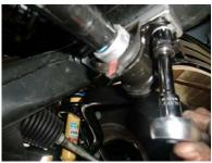
4. Install sway bar saddle brackets reusing the factory hardware.
