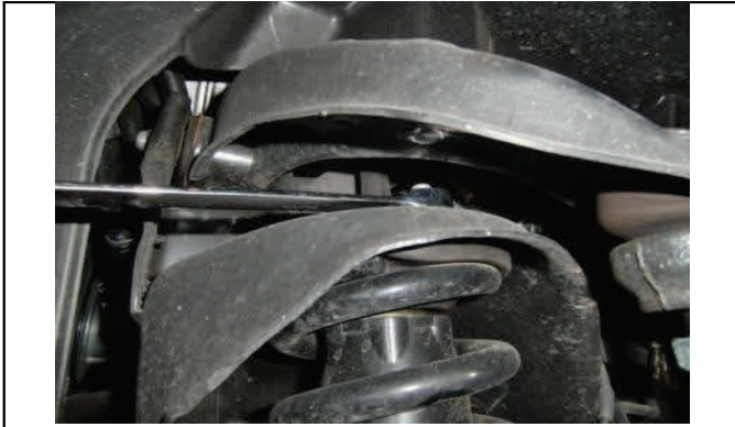
Remove upper strut mounting hardware
