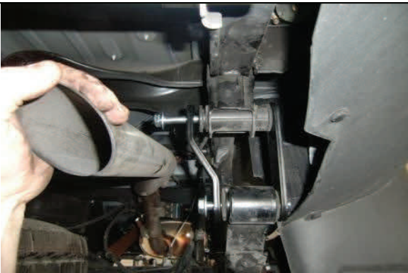
On passenger side, pull down on exhaust to gain access
