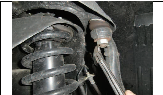
Remove cotter pin and upper ball joint
