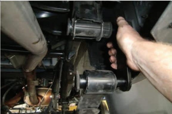
Lower axle and install new shackle bracket
