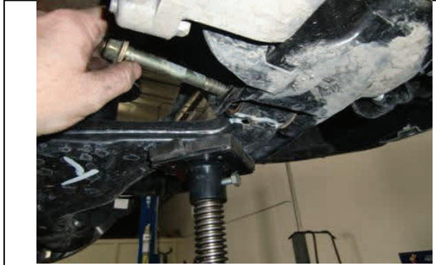
Support lower control arm, remove/replace bolts one at a time
