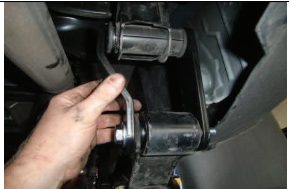
Attach new inner brackets and hardware
