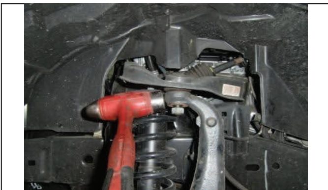
Strike spindle to break loose connection
