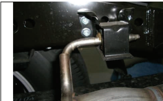
Unbolt rearmost exhaust hanger on frame
