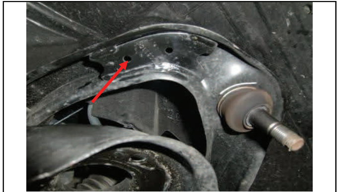
Drill 5/16 hole in upper control arm existing hole in as shown
