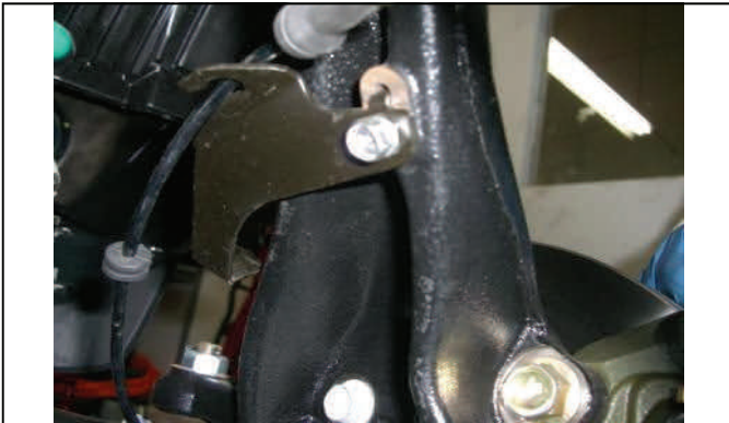
Disconnect ABS line bracket behind spindle
