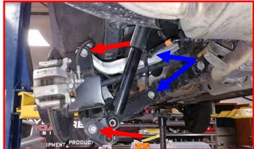
Loosen but do not remove the control arm hardware at the frame.
