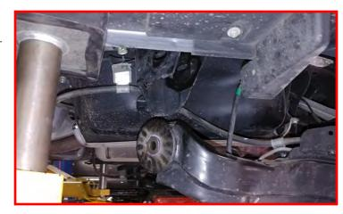
Once the control arm is lowered enough, remove the rear spring from the frame. Note the orientation of the lower spring pig tail and the locking tab on the lower isolator for reinstallation.
