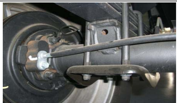
24. Support the rear axle, then remove the u-bolts and hardware.
