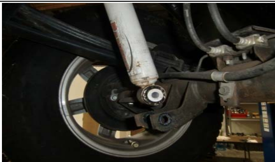
23. Disconnect the rear shock hardware and remove from the vehicle.
