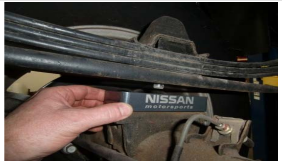
26. Lower the axle and install the lift block into position.
