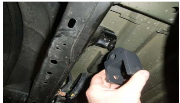
28. Install the provided shock extensions with the OE hardware.
