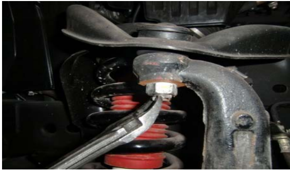
21. Install the new provided cotter pin.
