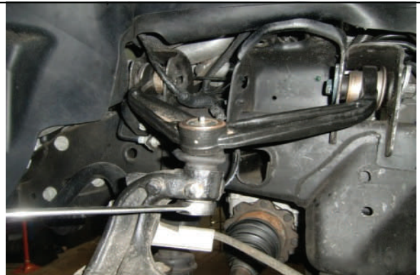
Loosen and remove upper ball joint nut.
