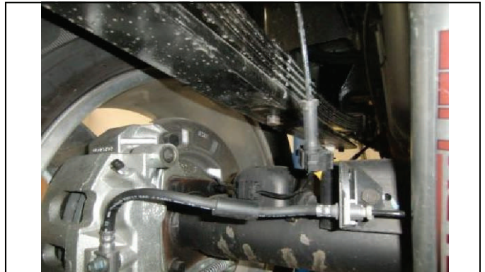
Carefully lower axle enough to install lift block
