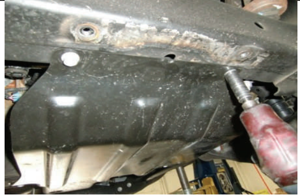
Reinstall front skid plate
