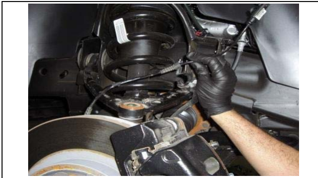
5. Unbolt the ABS bracket from the upper control arm.
