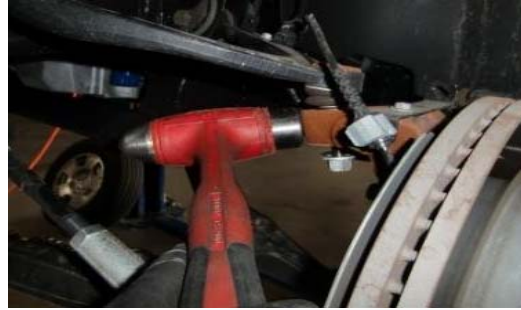
14. Strike the spindle as shown to break loose the ball joint, then disconnect.
