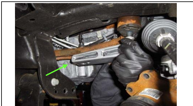
31. Re-install the bracket and attach the billet spacer as shown.
