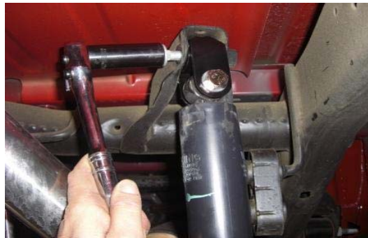
57. Re-install the shock with the extension attached and tighten.
