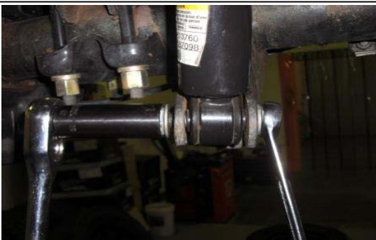
51. Disconnect and remove the rear shocks from the vehicle.
