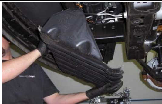
3. Remove the front plastic debris plate.
