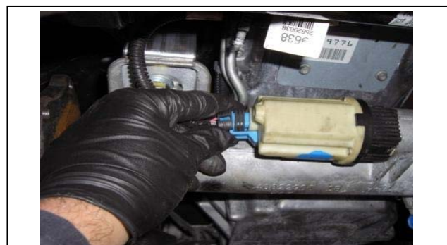
36. Re-connect the differential solenoid.
