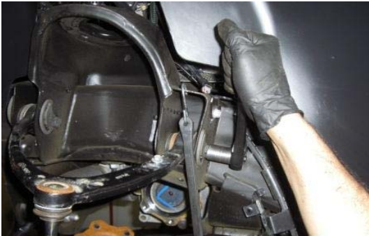
17. Unbolt the upper control arm marking the cam location.
