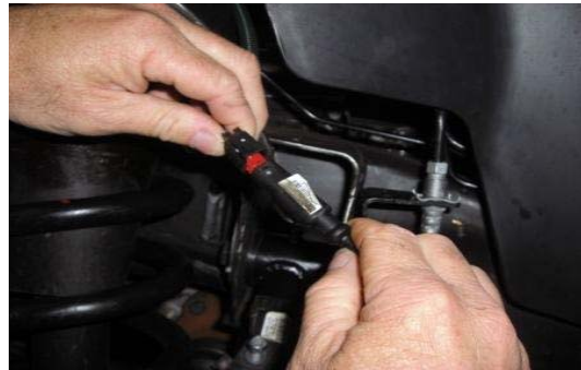
46. Re-connect the ABS plug near the frame.
