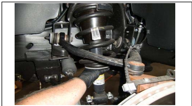
12. Remove the strut assembly from vehicle.
