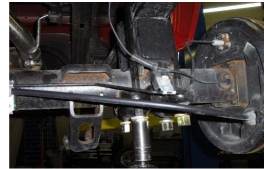
56. Raise the axle, align and attach the new u-bolts and hardware.
