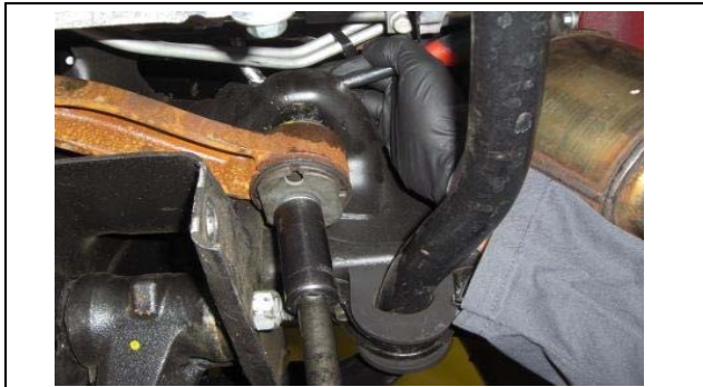
29. Remove the passenger side differential mounting bracket.
