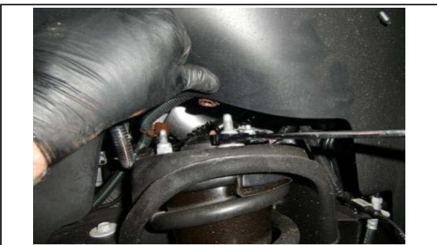
11. Remove the upper mounting nuts.
