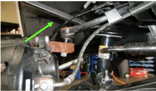
15. Use a pry bar to push down on the upper control arm, remove the nut.
