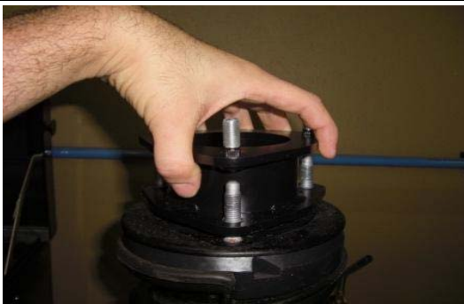
39. Place the new strut extension spacer onto the strut.
