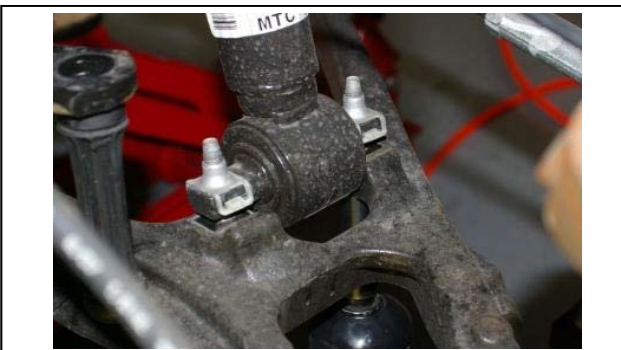
9. Remove the lower strut mounting hardware and the nut clips.
