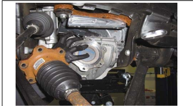
33. Position the differential into the vehicle, checking for clearance.
