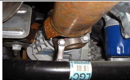
20. Disconnect the u-joint at the differential and slide back.
