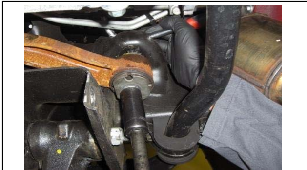
29. Remove the passenger side differential mounting bracket.
