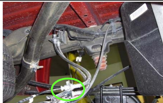
60. The differential brake line bracket may require bending up.
