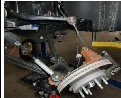
16. Carefully separate the ball joint from the spindle.
