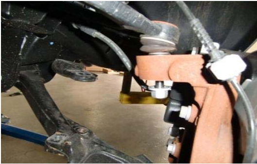
13. Loosen, but do not remove the upper ball joint nut.
