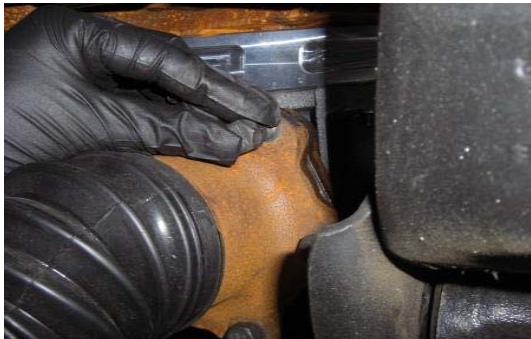
45. Re-attach the CV axles to the differential (6 bolts per side).
