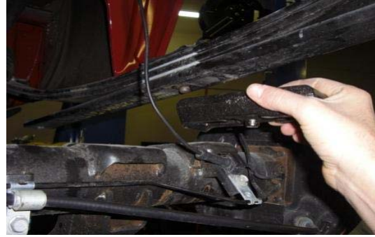
54. Lower the axle and remove the factory block, do not reuse .
