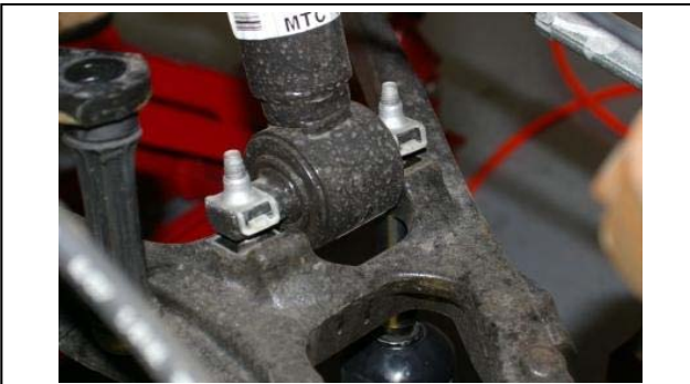
9. Remove the lower strut mounting hardware and the nut clips.
