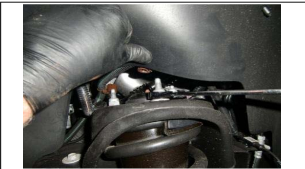
11. Remove the upper mounting nuts.
