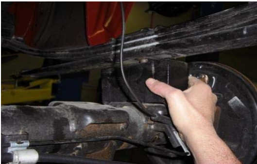
55. Lower the axle more in order to install the new lift block.
