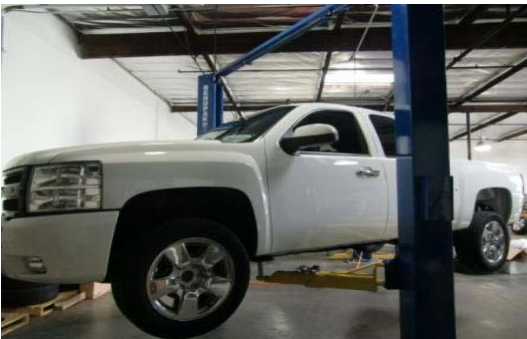
1. Raise the vehicle and support the frame with jack stands.
