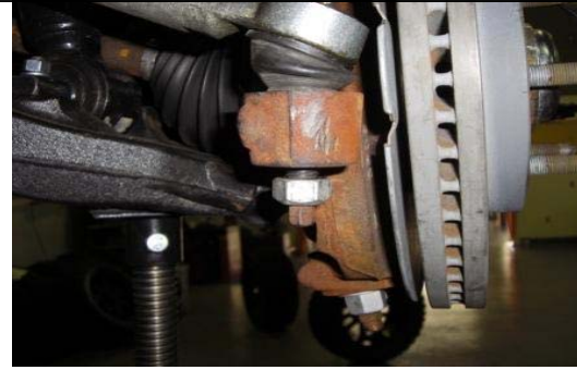
44. Connect outer tie rod end and sway bar end links and tighten.
