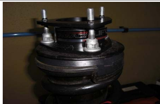
40. Attach and tighten with the OE hardware.
