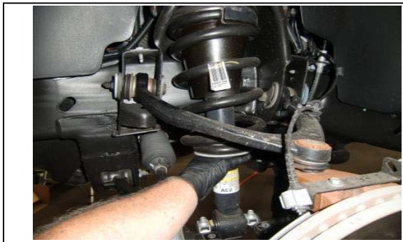
12. Remove the strut assembly from vehicle.
