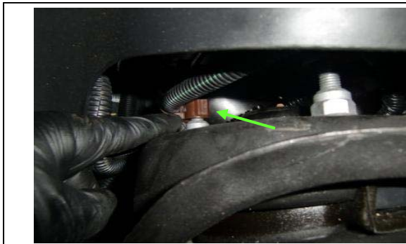
10. Remove the clips from on top of the upper strut mounting nuts.
