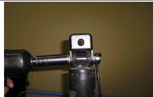
52. Install the shock extensions to the upper shock mount as shown.
