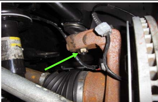
43. Raise spindle, attach upper ball joint, tighten, & insert cotter pin.
