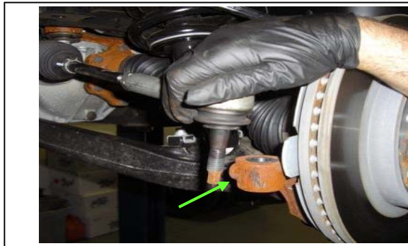
8. Strike the spindle with a hammer to break loose the tie rod.
