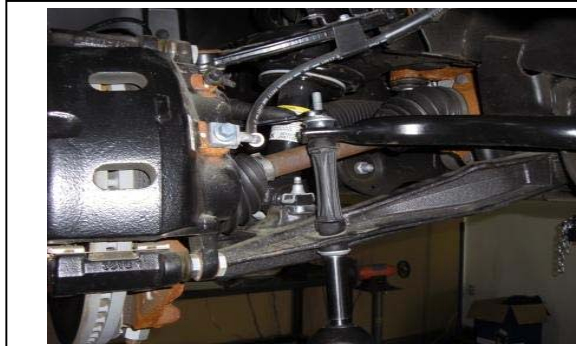
6. Disconnect and remove both sway bar end links.
