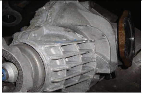
Use a grinder to remove material marked previously
