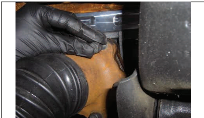
Reattach CV axles to differential (6) bolts and tighten
