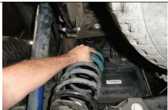
Lower axle and remove coil springs and isolators
