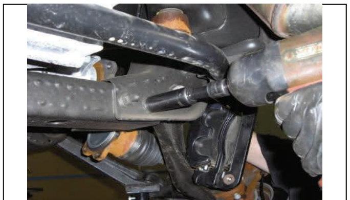
Unbolt rear cross member (4) bolts and remove
