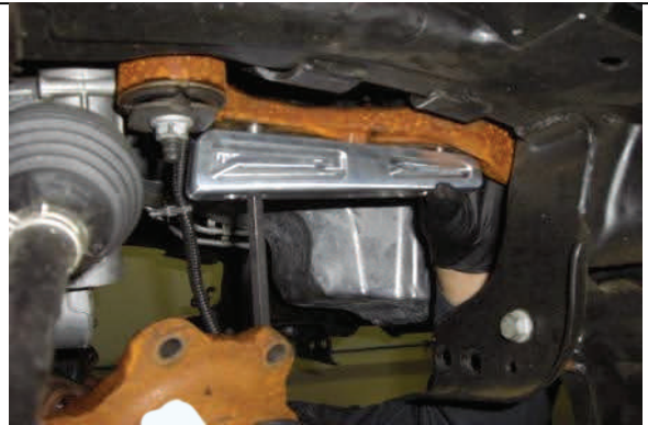
Attach passenger/driver side with socket head hardware
