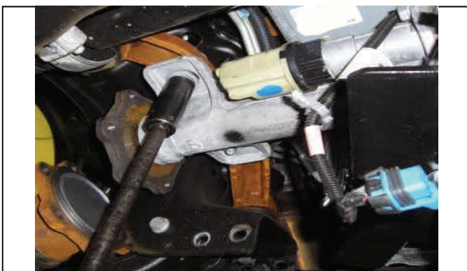
Support differential with jack and un-bolt passenger side
