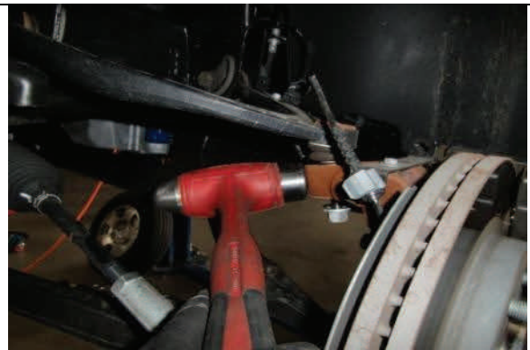
Strike spindle as shown to break loose ball joint, disconnect
