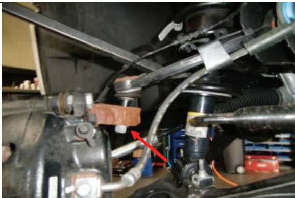
Use pry bar to push down upper control arm, remove nut
