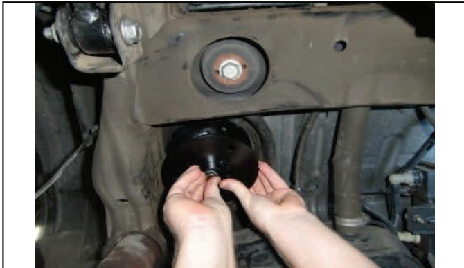
Attach coil spring spacer to nut plate and tighten
