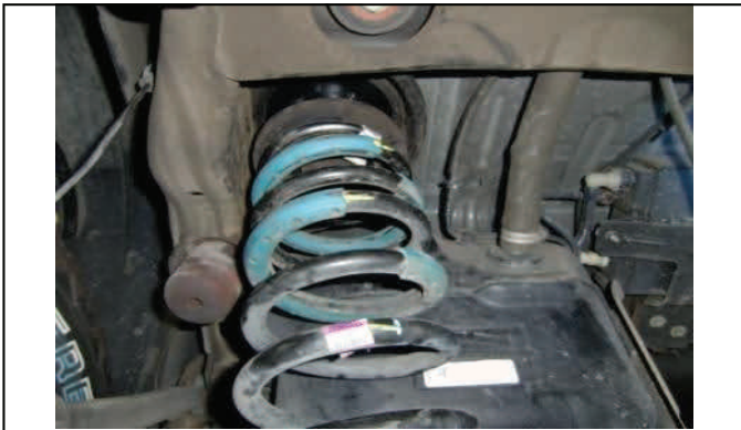
Reinstall isolators and coil springs and raise axle
