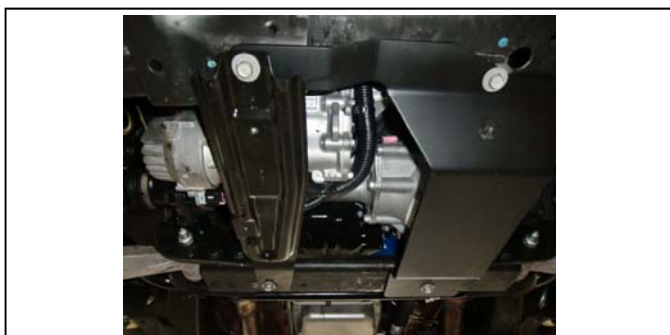
43. Re-attach passenger side sheet metal for air dam mount.
