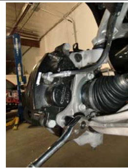
8. Remove caliper & secure to vehicle out of the way.
