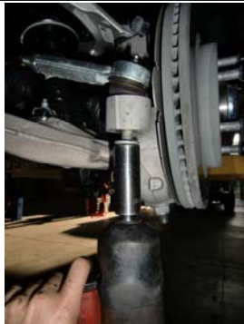
9. Loosen tie rod and remove from knuckle.
