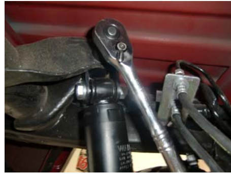
62. Once lower mount is tight torque the top shock mount.
