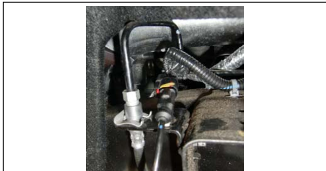
41. Reconnect ABS lines and attach in factory location.
