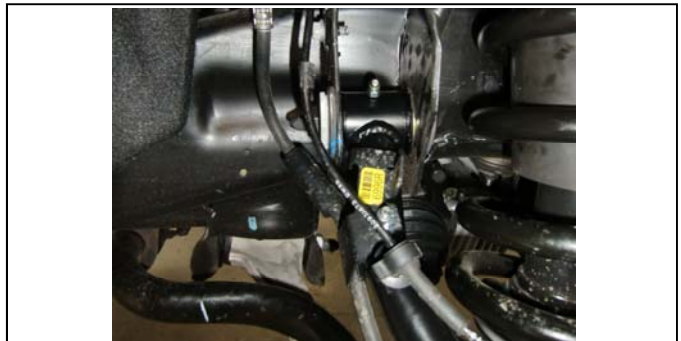
40. Reconnect brake line to control arm using new hardware.
