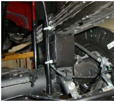
65. Using the zip ties provided attach the ABS line to the U bolt's
