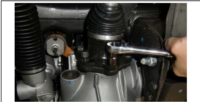
39. Reconnect Inner CV flange torque.
