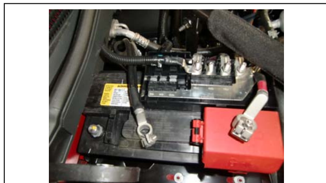
3. Disconnect battery connections.
