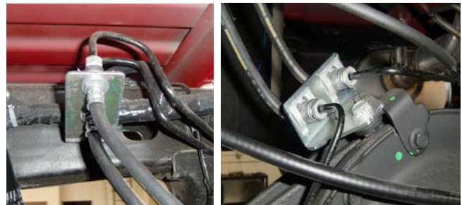
66. You may need to bend the upper and lower brake line brackets to allow enough slack in the line at full droop.
