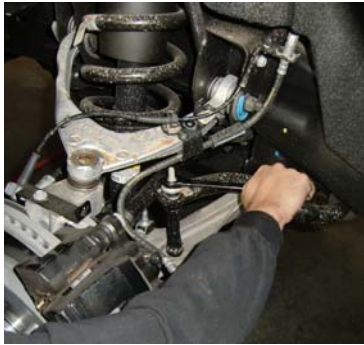
7. Disconnect sway bar & swing it out of the way.
