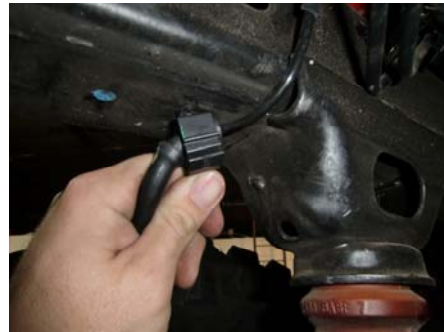
64. Re-clip the ABS line back into place.
