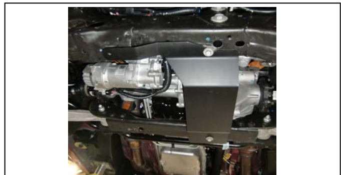
42. Install new ReadyLIFT skid plate.
