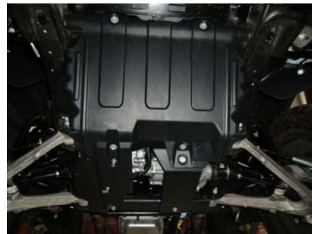
48. Use provided hardware to complete install of the air dam.
