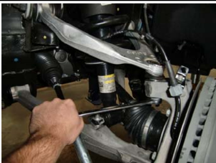
11. Loosen & separate ball joint from knuckle.
