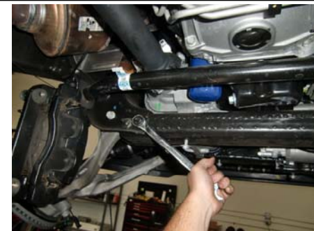
20. Loosen and remove cross member.
