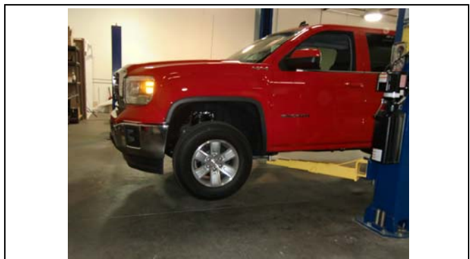
2. Raise vehicle and support vehicle to perform work.
