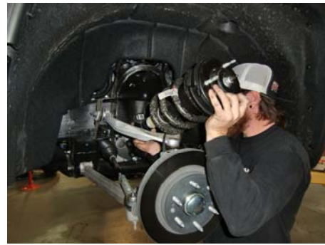
14. Remove strut from vehicle. Repeat 5-14 for other side.
