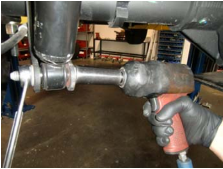
61. Install shock into lower mount and tighten.
