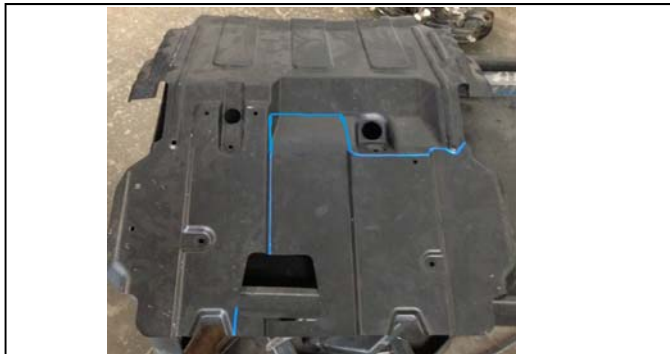
45. Cut lines marked on air dam.
