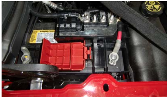
67. Reconnect Battery and the installation is complete.
