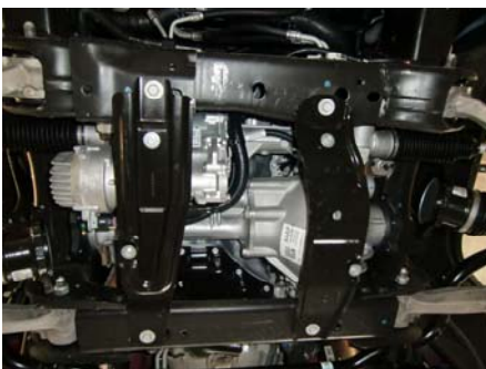
19. Remove plastic air dam tin mounting brackets.
