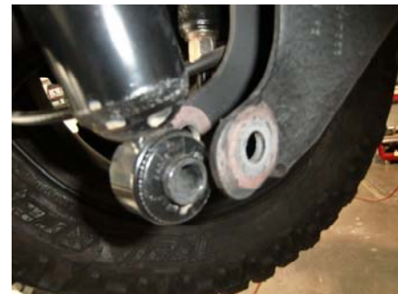
52. Support the axle, remove the shock from the lower mount.
