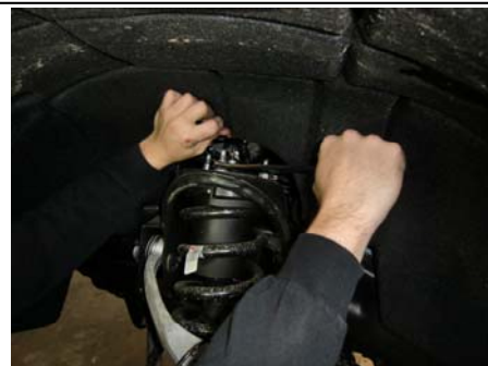
12. Remove nuts from the top of the struts.
