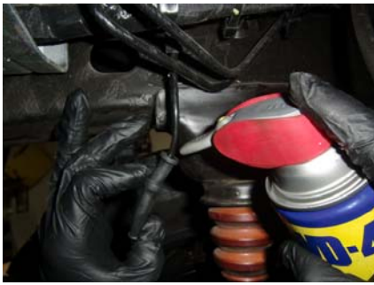
63. Lubricate the ABS line and slide rubber sleeve up to allow the wire to be re-installed in to frame clip.
