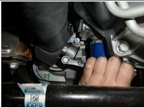
17. Loosen and remove front drive shaft bolts and straps.
