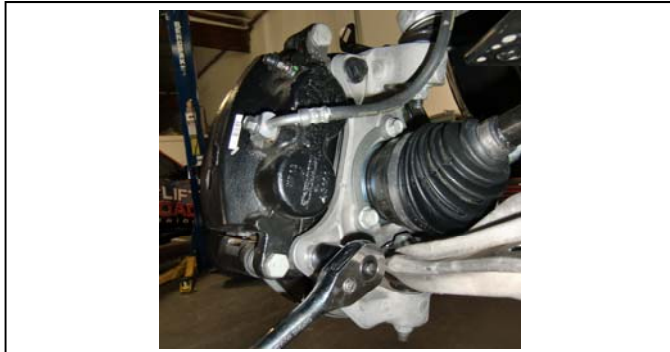
37. Re-attach caliper & torque. Repeat 29-37 on other side.
