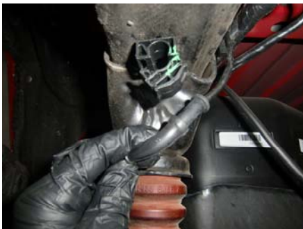
51. Unhook ABS line located on the rear of the frame.
