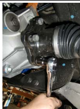
10. Remove bolts from inner CV drive flange.
