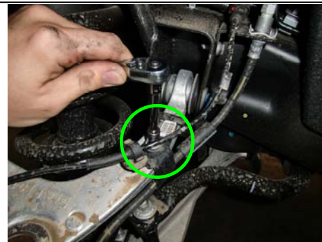
6. Unbolt brake line from upper control arm, unclip the ABS line.
