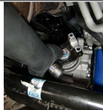
18. Slide drive the shaft back and out of the way .
