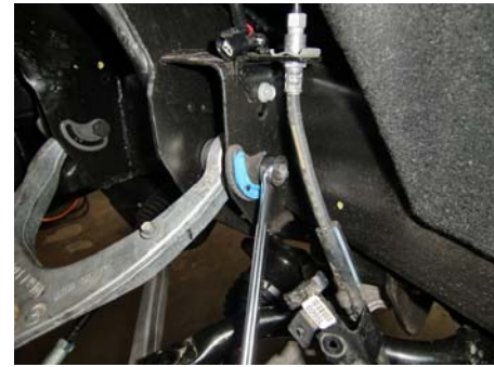
16. Remove hardware and arm. Repeat 15 & 16 on other side.
