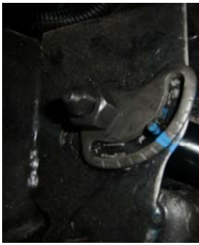
15. Mark alignment cams & note direction/location of hardware.
