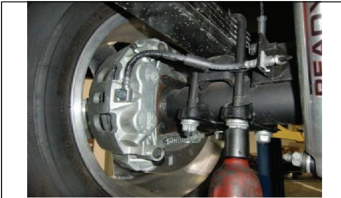
Loosen and remove u-bolt hardware
