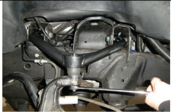
Connect upper ball joint to spindle
