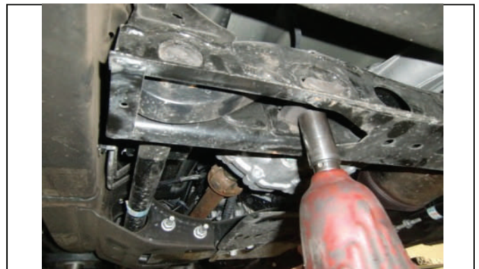
Remove torsion bar adjuster bolt. It will be reused.
