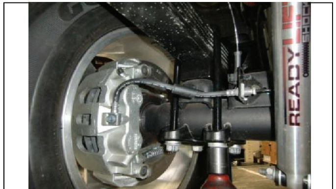
Torque u-bolts with vehicle on ground and re-clip ABS wire
