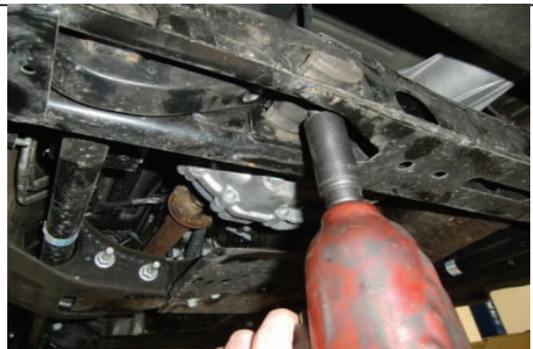
Adjust torsion bars to approx ride height
