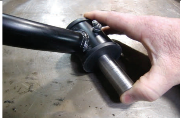
Assemble bushing halves and insert crush sleeves
