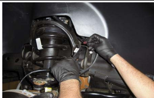
4. Disconnect the ABS sensor at the frame.
