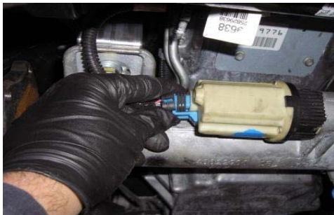
19. Unplug the differential solenoid.
