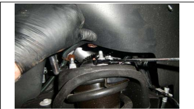
11. Remove the upper mounting nuts.
