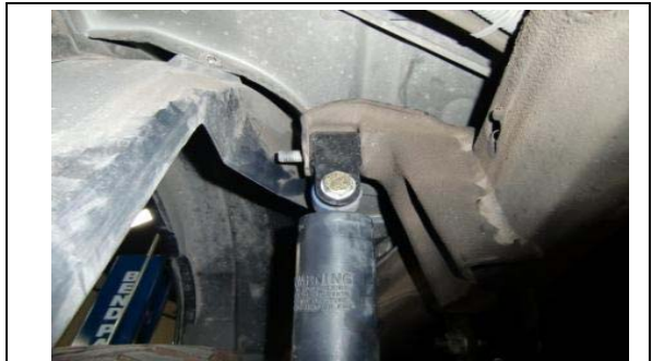
70. Re-install the shocks with extensions as shown and tighten.
