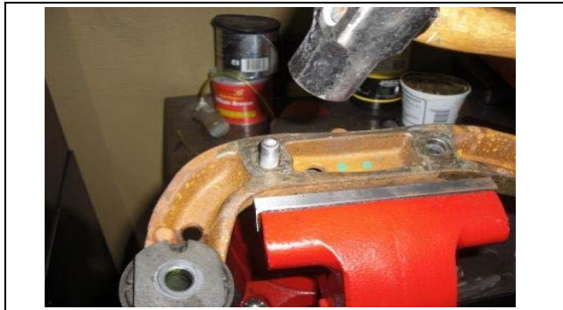
30. Secure in a vise and remove the mounting studs with hammer.
