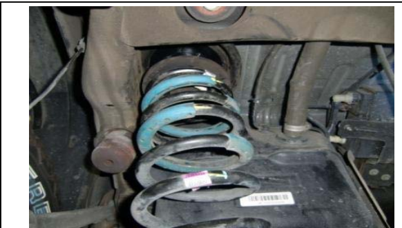
69. Re-install the isolators and coil springs and raise axle.
