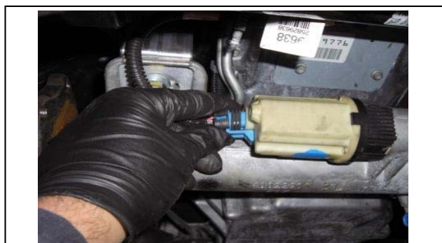
36. Re-connect the differential solenoid.
