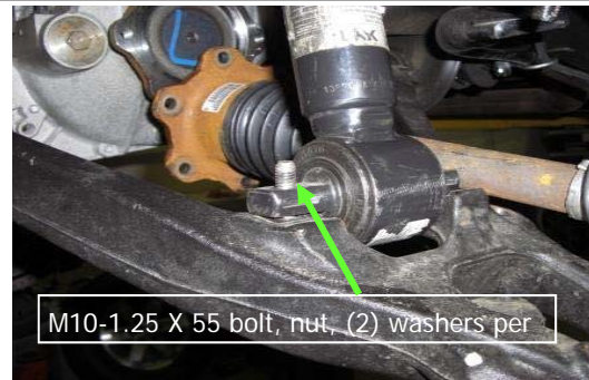
42. Attach the lower strut mount with new shorter hardware, no clips .
