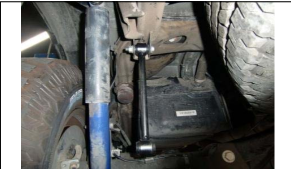
71. Install the new longer sway bar end links and tighten.
