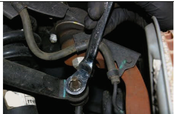
Disconnect and remove sway bar end links
