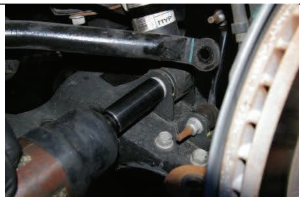
Remove lower strut mounting hardware
