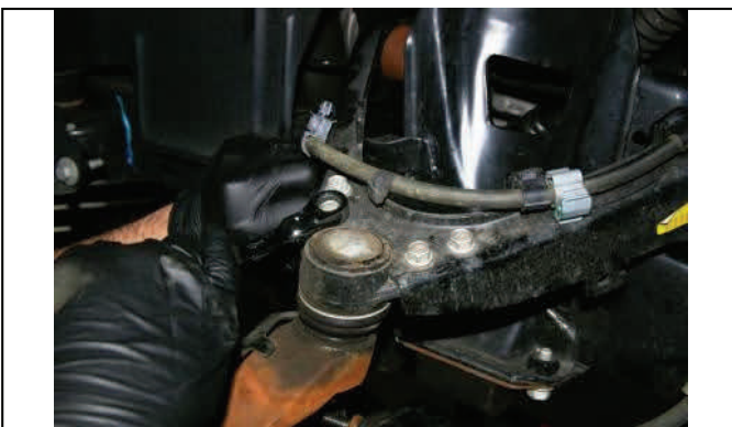
Unbolt upper ball joints from upper control arm
