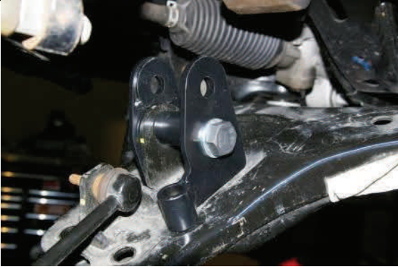
Assemble lower strut extension brackets as shown
