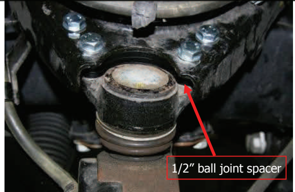
Lift suspension, insert upper ball joint spacer w/ new hardware
