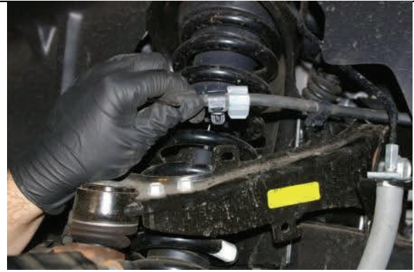
Unclip brake lines from upper control arms
