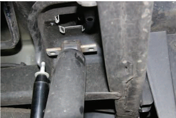
Support axle and remove upper shock mounting hardware
