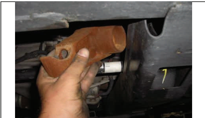
Remove OE torsion key
