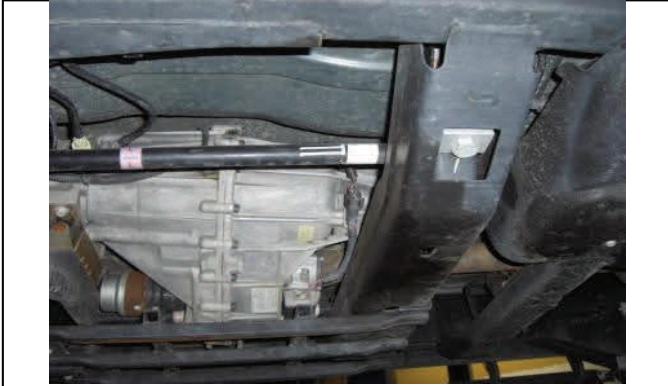
Raise and support vehicle on jack stands, locate torsion bars
