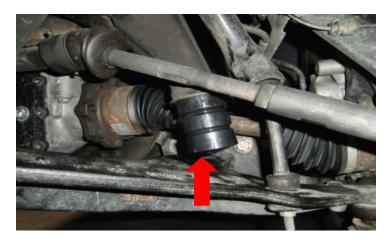
Use the torsion bar unloading tool, load the torsion bar enough to install the cross pin. DO NOT pull it through with your fingers.
