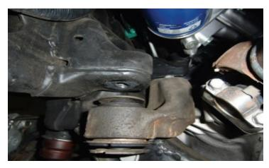
Install the ReadyLIFT differential spacers between the differential cradle and frame using the provided bolts and laser cut washers. Use factory flange nuts. Torque all to 95 ft-lbs.
