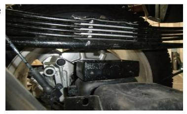
Raise the axle with the ReadyLIFT block installed to the leaf pack. Install the provided U-bolts and hardware. Only snug the U-bolts up enough to hold the axle in place. Repeat all steps on the passenger side. Final torque will be done when the vehicle is on the ground.
