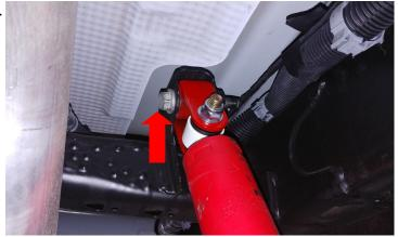
Reattach the shock to the axle using factory hardware. Hand tighten only, final torque will be done when the vehicle is on the ground.
