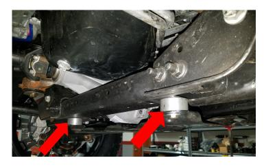
Trim the plastic gravel guard. Cut a slot just large enough for a 3/8 bolt to slide freely, on the lower mount that connects the gravel guard to the skid plate. Use the provided spacers large washers and bolts to attach at the lower mount. Hand tighten only. Use the factory hardware to attach the top of the gravel guard in its original position. Torque all bolts to 25ft-lbs.
