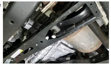
Factory torsion key part# 84634344 Screw the torsion key adjuster bolt in until you reach the torsion key and is snug. Turn the adjuster bolt in one full revolution.
