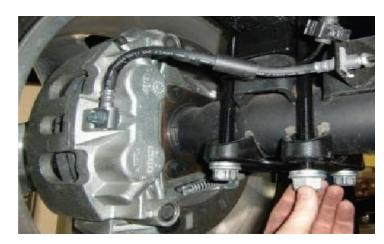
Install the shock extension using the provided M14 bolts, washers, and nuts to the top of the factory shock.
