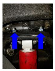
Measure and record the torsion key adjuster bolt length. Remove the torsion bar adjustment bolt.
