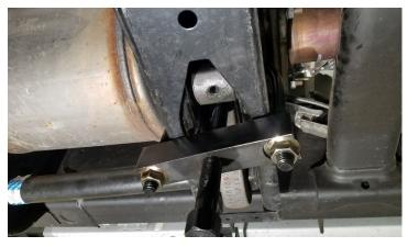
Factory torsion key part# 84461807 reuse factory adjustment bolt.
