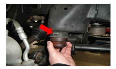
Install the ReadyLIFT bump stops. Use a soapy water solution to aid in install. You may need to use the lower control arm and a jack to "press" them into place.
