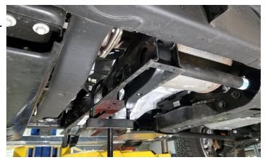
Remove the gravel guard and skid plate. Support the differential with a suitable jack.
