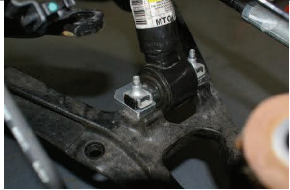
Install lower strut spacer and tighten,
