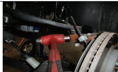
Strike spindle with hammer to loosen ball joint
