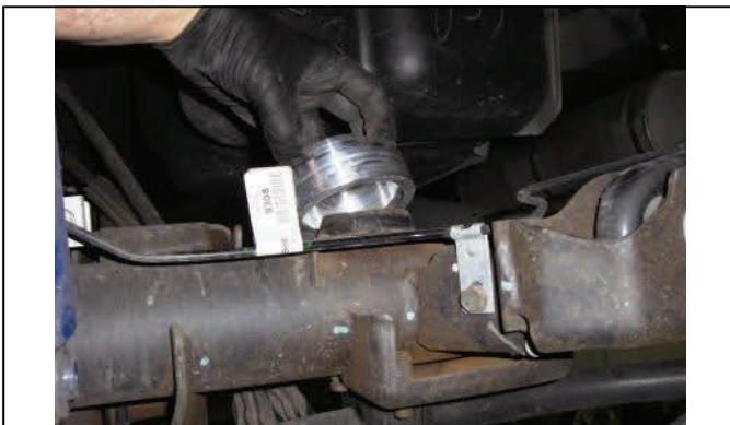
Place ReadyLIFT spacer on axle mount
