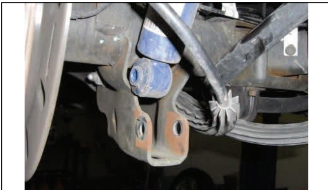
Disconnect Lower shock mounts
