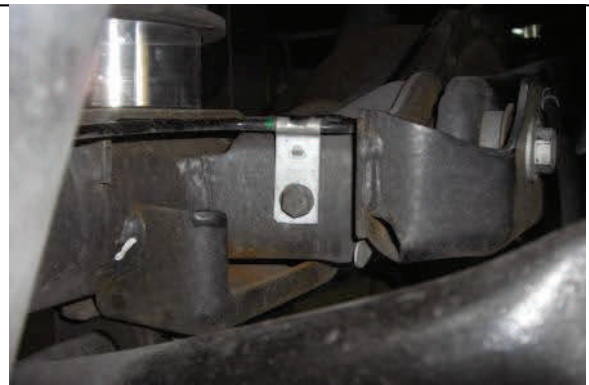
Unbolt dr/pass brake lines on axle
