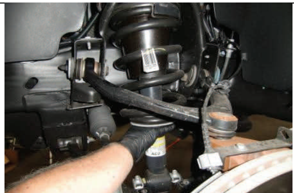
Remove entire strut assembly from vehicle.
