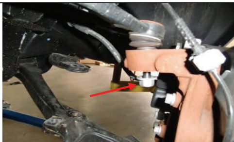
Support suspension loosen upper ball joint nut
