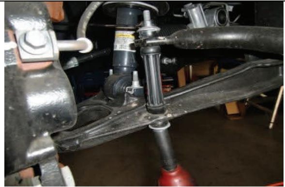
Disconnect dr/pass sway bar end links
