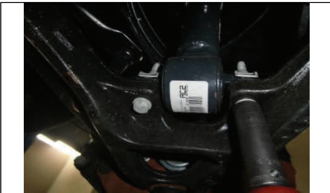
Remove lower strut mounting bolts
