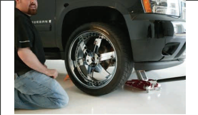
Raise and support vehicle frame on jack stands
