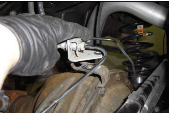
Disconnect brake lines at top of differential
