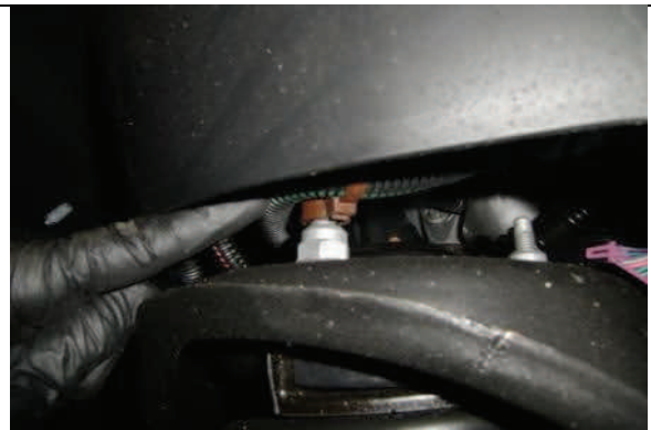
Pry up ABS retaining clips from upper strut mounting nuts
