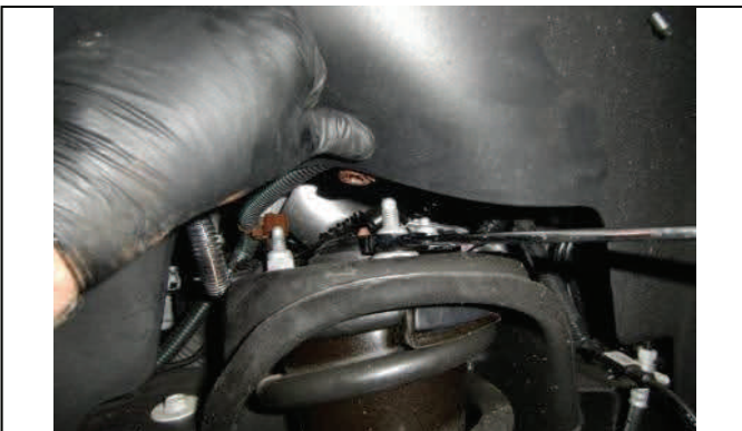
Remove upper strut mounting nuts
