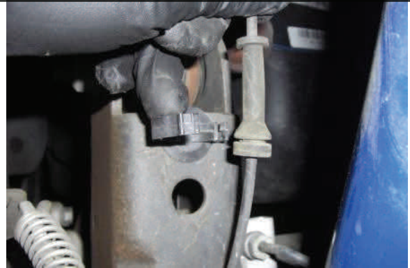
Unclip ABS lines at upper trailing arm
