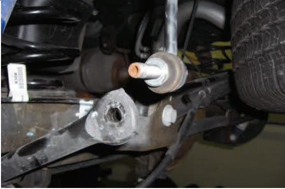
Support axle with jack and disconnect sway bar end links
