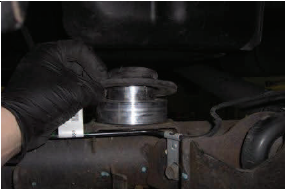
Refit OE rubber isolator on top of billet spacer
