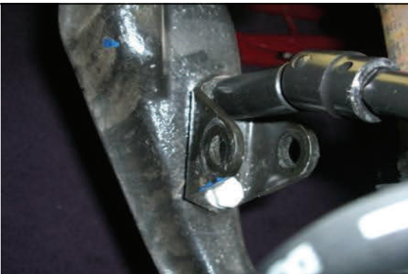
66-3050 shock extensions will replace the OE brackets
