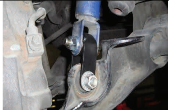
66-3000 Install front lower shock extensions and hardware
