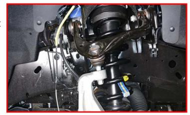
Install the tie rod end to the knuckle using the factory hardware. Torque to 45 ft-lbs.
