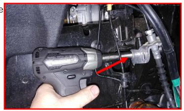
Remove the brake line bracket and ABS harness on the knuckle.
