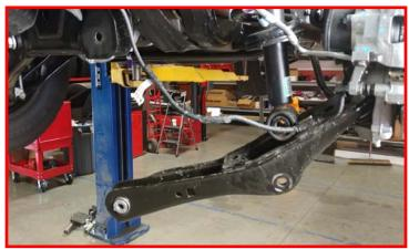
Locate the ReadyLIFT strut spacer. Install using the provided M10 - 1.5 flange nuts. Torque to 30 ft-lbs. Install the completed strut assembly into the frame using the provided M10 - 1.25 flange nuts. Do not tighten at this time.
