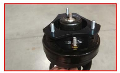
Raise the lower control up to the strut. Install the strut hardware. Do not tighten at this time. Raise the lower control arm up to the frame and install the control arm hardware. Do not tighten at this time. Install the ABS harness clips to the lower control arm.
