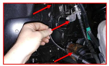
Remove the brake line bracket at the frame rail.
