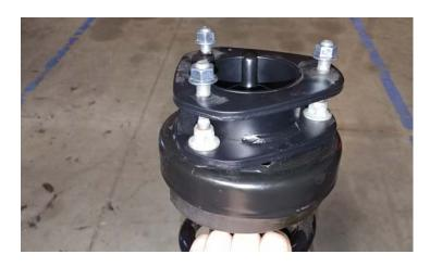
Install the completed strut assembly to the frame using the provided M10 -1.25 Flange nuts. Do not tighten at this time.
