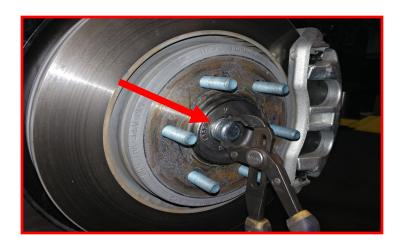
Remove the CV axle nut.
