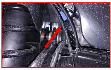
Disconnect the electrical connector and remove the wire from all other points on the frame. Picture is of the top of the inner fender well plastic showing the harness clip for the electrical connection. This can be accessed from under the hood or reaching up behind the plastic. Remove this clip from the plastic liner as it will need to be relocated in a later step.
