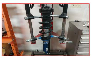
1.5" and 2.5" kit top extension: Install the factory nuts onto the strut hat studs running them down until they bottom out. Using a suitable cutting tool, cut the studs off just above the nut. Remove the nuts and clean any off any burs. Paint the exposed metal with a quality rust preventative paint.
