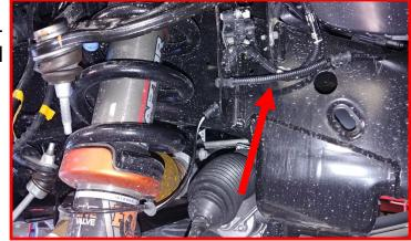
Disconnect the electrical connector and remove all clips from the frame rail.
