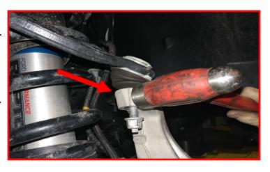
Support the lower control arm with a suitable jack. Loosen but do not remove the lower control arm bolts at the frame rail. Remove the lower coil over bolt.
