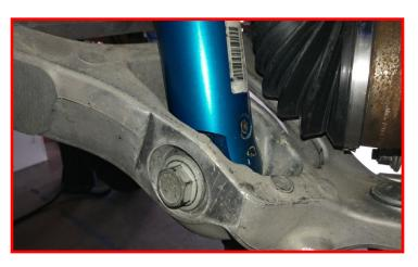
Raise the upper control arm up. Mark the frame in the center between the pocket walls 3/4" down from the edge.
