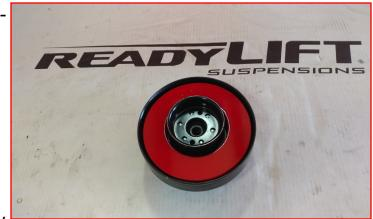
2.5" kit Pre-load spacer: Install the factory top hat onto the strut assembly 180 degrees from the factory orientation using the previous marks made as a guide. This is very important for spring to control arm clearances once the strut assembly is installed back into the vehicle.
