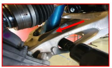
Remove the upper strut mount at the frame and remove the strut from the vehicle. Mark the top hat and lower spring perch in relation to the strut body. This is very important to keep the spring to upper control arm clearances for full droop.
