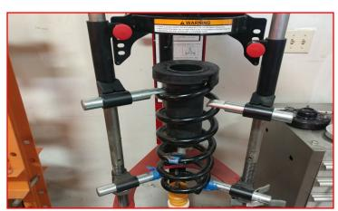
2.5" kit Pre-load spacer: Install the Ready-LIFT spring spacer into the top hat.
