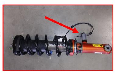
2.5" kit Spring spacer: Remove the factory top hat. Pull the rubber isolator and dust shield out and replace onto spring.
