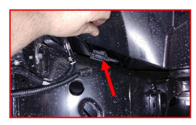
Driver side, locate the electrical harness on the coil over and follow it up onto the frame rail and into the engine bay. The wire follows the ABS harness.
