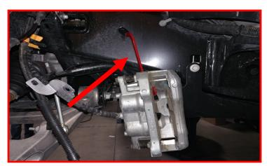
Loosen but do not remove the upper ball joint nut at the knuckle. Strike the ball joint boss with a dead blow hammer to dislodge the taper. Remove the ball joint from the knuckle. Support the knuckle as to not let it fall to protect the vacuum hub. Loosen but do not remove the upper control arm bolts at the frame rail.
