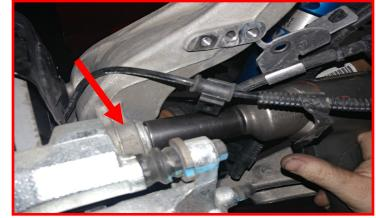
Use a suitable hanger, hang the caliper out of the way. Never let the caliper hang from the rubber line. Remove the rotor from the hub.
