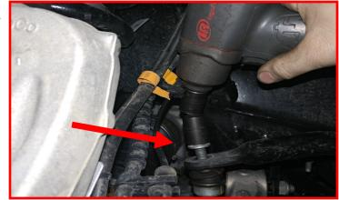
Remove the CV axle nut cover.
