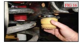
Install the ReadyLIFT® bump stop spacer and factory bump stop mount to the frame using M8 x 70 mm bolt and washer. Torque to 5 ft-lbs.
