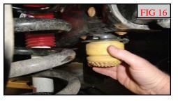
Install the ReadyLIFT® bump stop spacer and factory bump stop mount to the frame using M8 x 70 mm bolt and washer. Torque to 5 ft-lbs.
