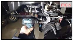
Remove the lower shock from the axle mount. (Fig 7)
